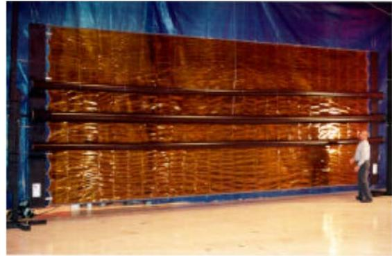
(b) Teledesic Inflatable Solar Array
