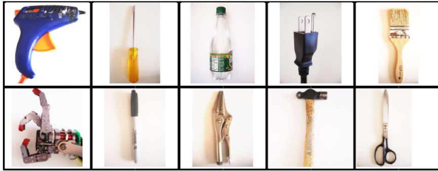
Figure 2.3: Kemp and Edsinger 45 demonstrated the tip detection on these tools (hotglue gun, screwdriver, bottle, electrical plug, paint brush, robot finger, pen, pliers, hammer, and scissors). The method performed best on the tools with sharp tips.
