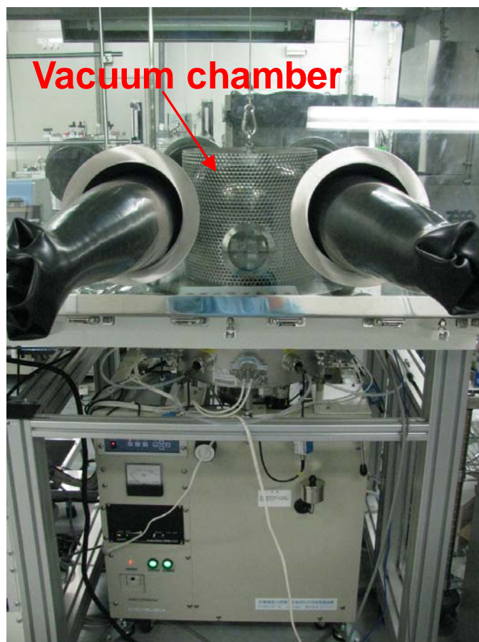
Fig.2.3 Vacuum chamber contained within a glove box.
