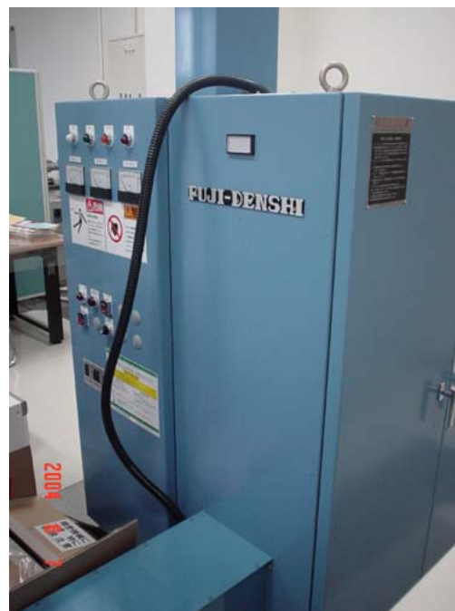
Fig 2.3-4 Power supply for induction heating device.
