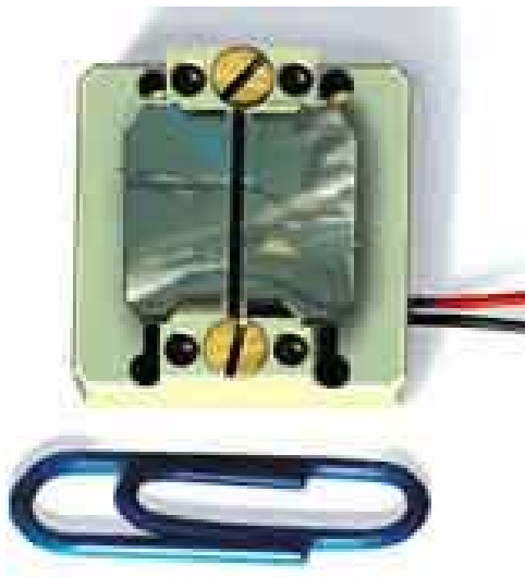
Fig.27 Adjustable piezo-electrically-driven slit.
