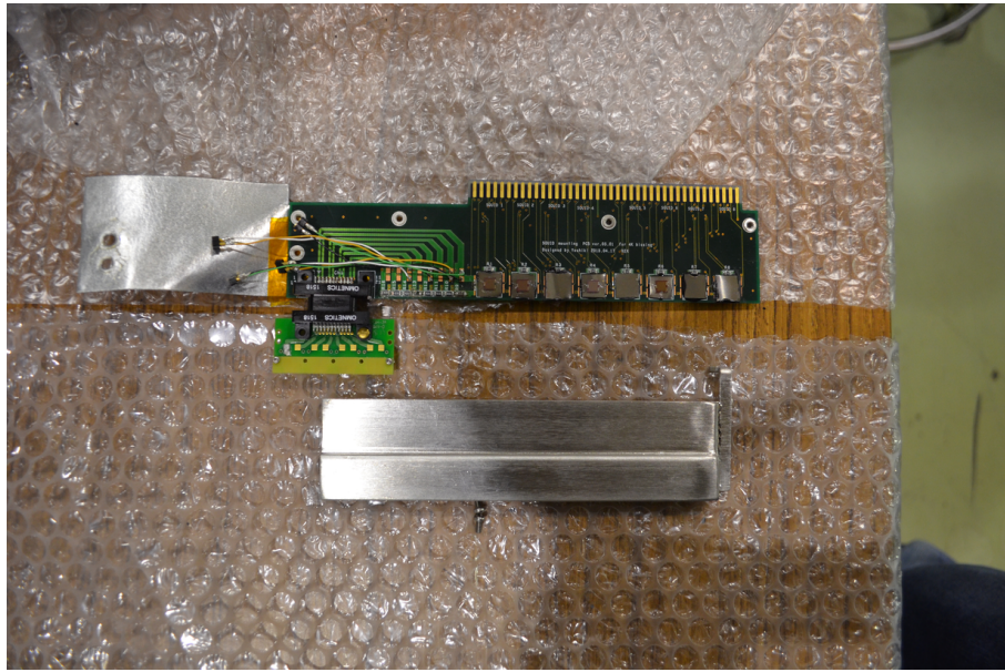
Figure 8.4: SQUID mounting board. We place eight SQUID chips on the board.
