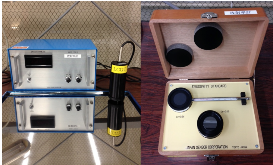
Figure B.1: Measurement system and calibration samples.
