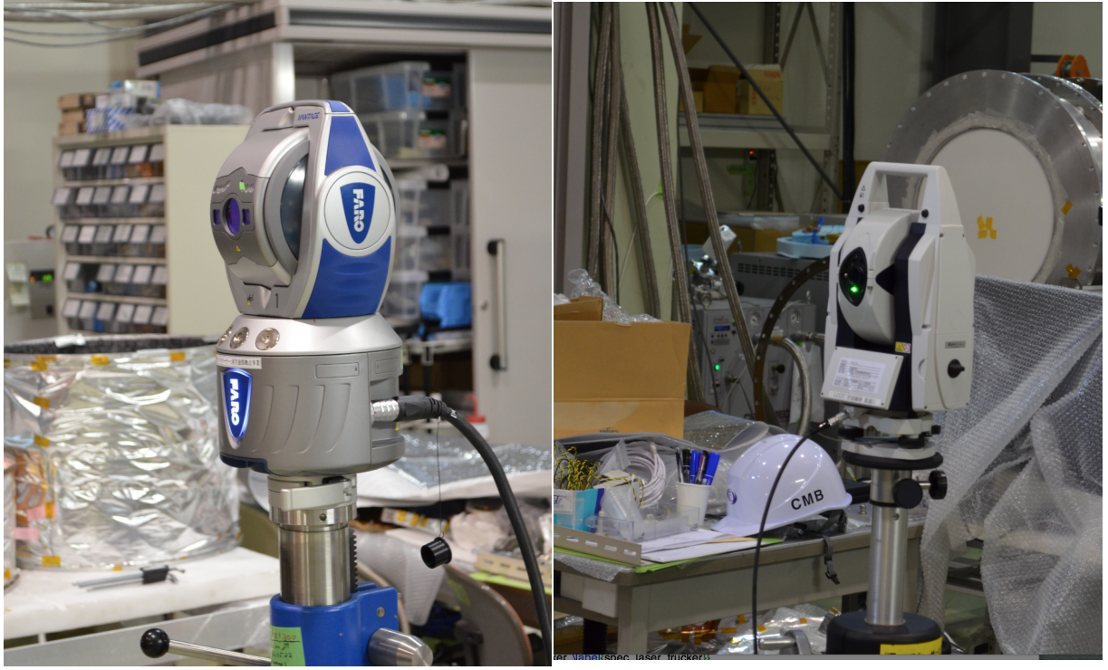
Figure 6.5: Laser trackers. (Left) FARO Laser Tracker Vantage. (Right) Leica AT401.
