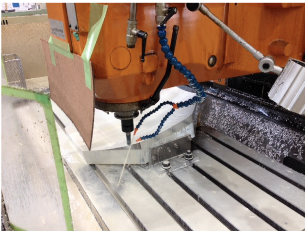
Figure D.2: The milling machine with a ball end mill.
