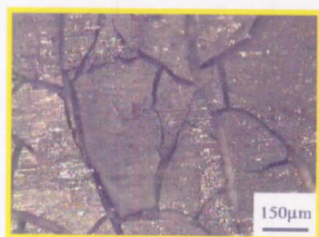
(a) Bonding layer surface (with p fiber printed)
