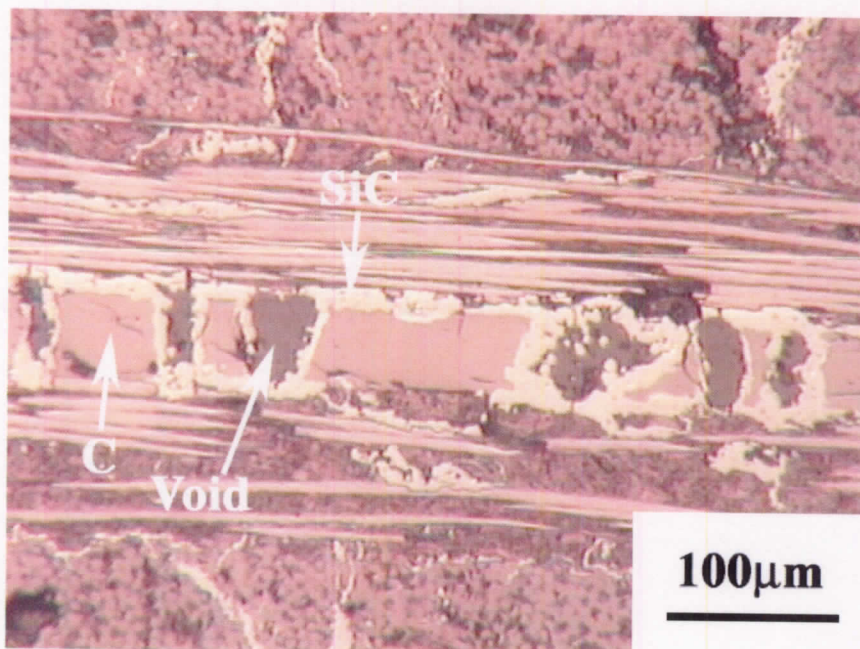
Fig.4-8 Cross sectional views of Hybrid bonding layer formed by Direct hybrid bonding. (Bonding thickness, h=50 \mu\text{m} )
