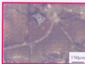
(b) Bonding layer surface (with non printed)
