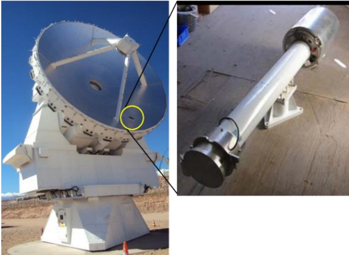
Figure 2-1 The ALMA ACA 7-m antenna and optical pointing telescope. Optical pointing telescope is mounted on buck up structure of the main reflector antenna which position indicates as circle.
