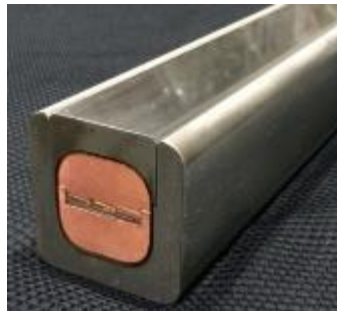
Fig. A.1.2 100 kA-class HTS conductor for helical coils of FFHR-d1
