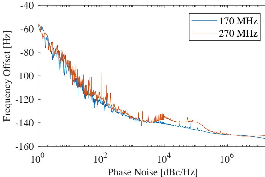
Figure 5.4: Phase noise at sampling frequencies used for direct sampling, 172 MHz and 270 MHz.
