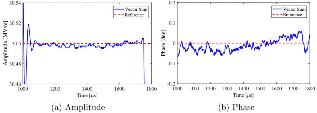
Figure 3.13: Flattop of vector sum of eight cavities operated in master-slave configuration.
