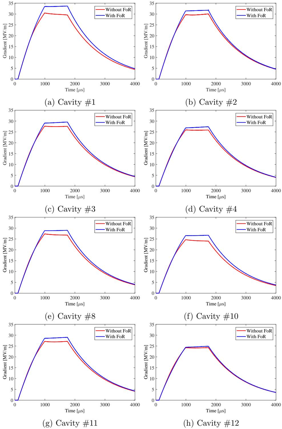
Figure 6.16: Cavity gradients of all eight cavities without and with filling on resonance method.
