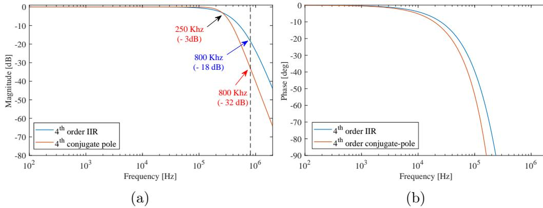
Figure 2.11: Comparison of fourth-order IIR filter (four first-order IIR filters connected in series) and fourth-order conjugate-pole IIR filter (two second-order conjugate-pole filters connected in series). The bandwidth of both filters was set to 250 kHz.
