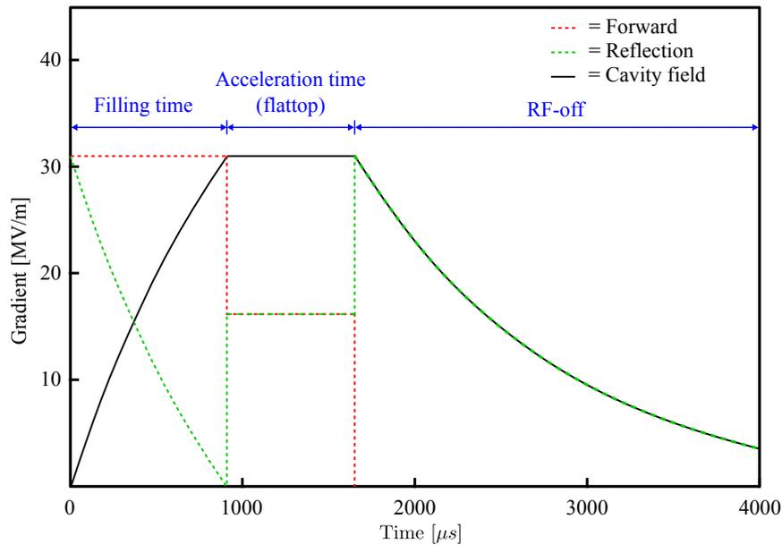
Figure 2.17: Typical RF forward pulse, reflection, and cavity field signals when there is no beam. The pulse signal consists of the filling time and beam acceleration time.
