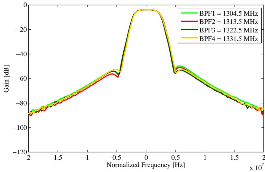
Figure 4.9: Frequency response of single filter. The filter frequencies are normalized.
