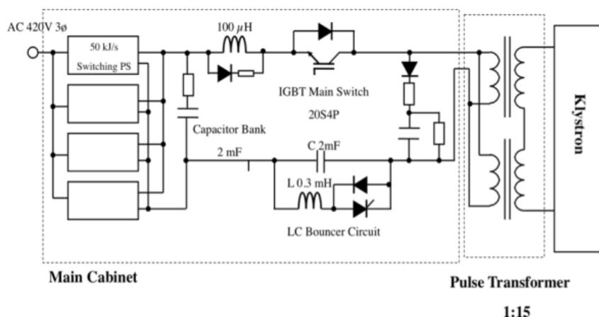
Figure 6.15: Simplified schematic of STF modulator. [43]
