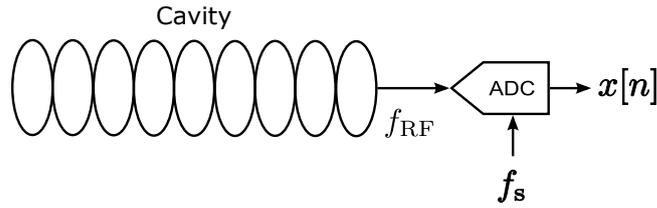
Figure 5.1: Front-end for direct sampling technique. The signal from the cavity is fed directly to the high-speed, wide-bandwidth ADC.  $f_{RF}$  is the input signal,  $f_s$  is the sampling clock, and  $x[n]$  is the sampled signal.
