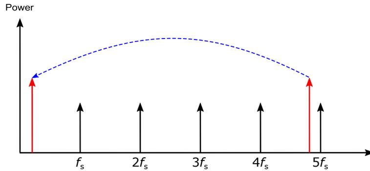
Figure 5.2: Direct sampling technique will translate the sampled signal to the first Nyquist band.
