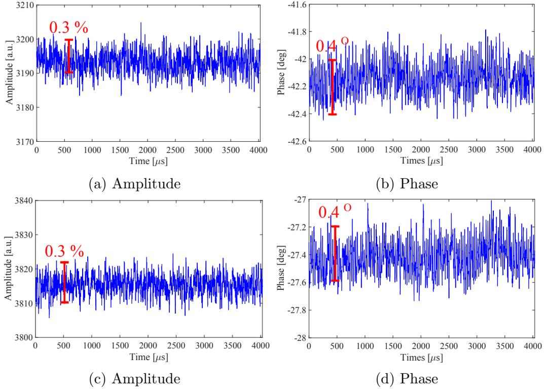
Figure 5.10: Amplitude and phase of (a) and (b) MO and (c) and (d) LO detected by direct sampling with the same sampling clock.
