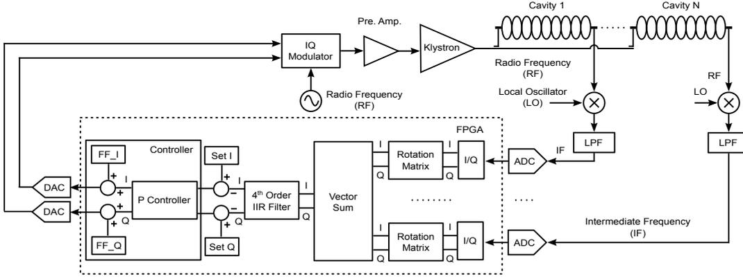
Figure 2.1: Simplified schematic of digital LLRF control system configuration with  $N$  cavities. Each component of the feedback loop is explained in the text.
