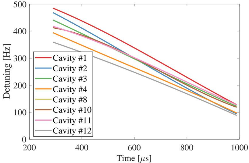
Figure 6.18: Detuning patterns of eight cavities after they were fitted with third-order polynomial fitting during the filling time.
