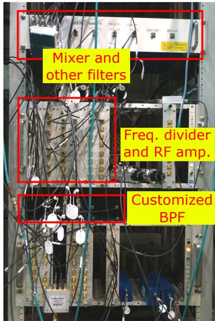
Figure 4.8: Photograph of setup for LO generation for multi-IF technique.
