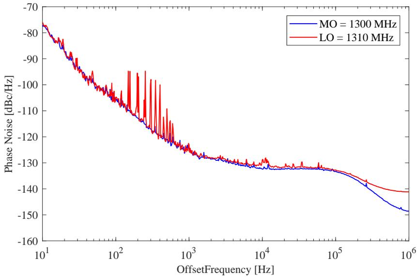
Figure 3.8: Phase noise of MO and LO. For the MO, the estimated jitter is 56 fs, which corresponds to 26 mdeg. For the LO, the estimated jitter is 60 fs, which corresponds to 28 mdeg.
