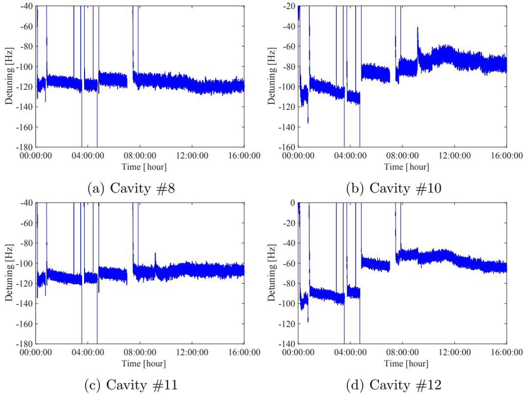
Figure 6.7: Detuning of cavities #8, #10, #11, and #12 at the end of the RF pulse. Data were taken for 16 h, as indicated on the time axis of the detuning plot.
