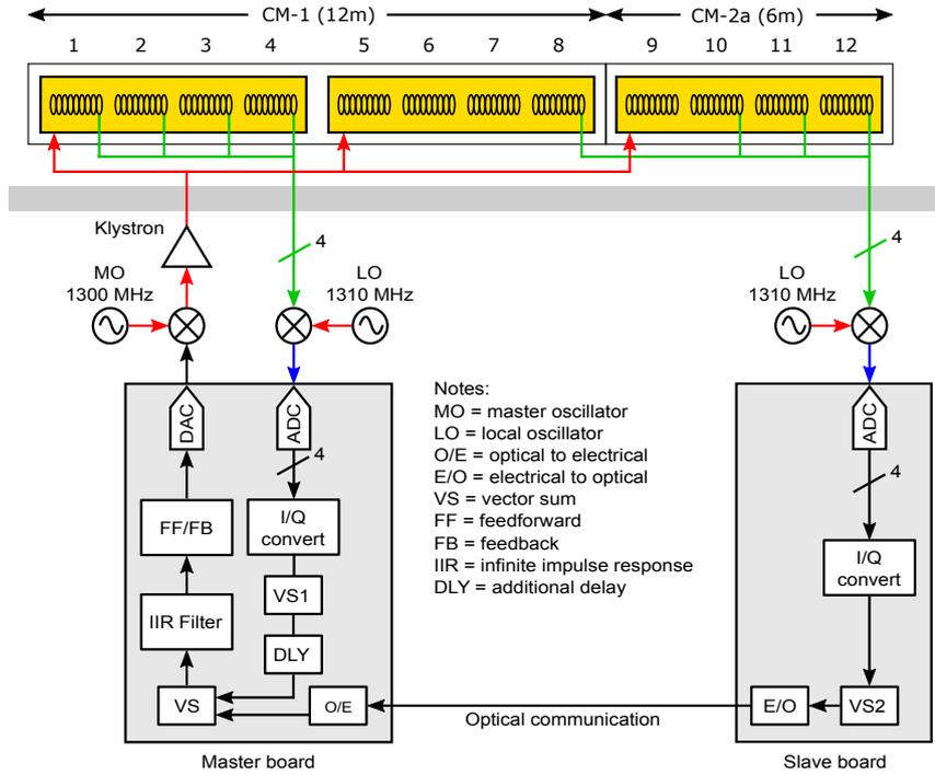
Figure 3.1: Simplified diagram of minimum setup of digital LLRF control system with master-slave configuration at STF-KEK. VS1 is the partial vector sum of the cavities connected to the master board. VS2 is the partial vector sum of the cavities connected to the slave board.
