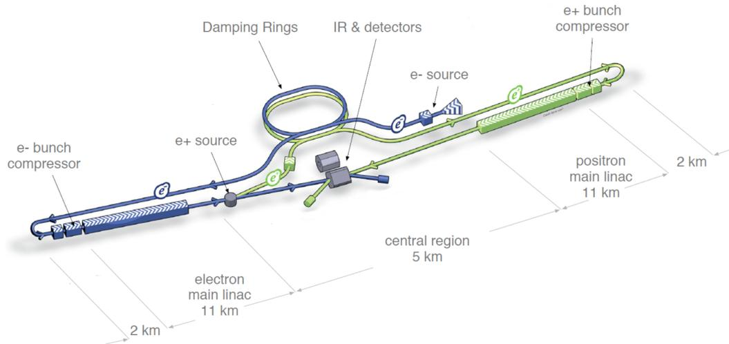
Figure 1.1: Layout of ILC showing all the major subsystems [1]. The total length is approximately 31 km.
