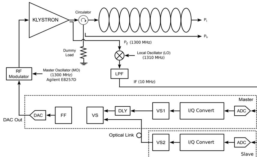
Figure 3.4: Measurement setup used to estimate the delay time introduced by the optical link communication and to estimate the loop delay. Only the forward signal is used in the evaluation. Two ADCs on the master and slave boards are fed with the same signal. The forward signal is chosen because it has a sharp edge at the end.
