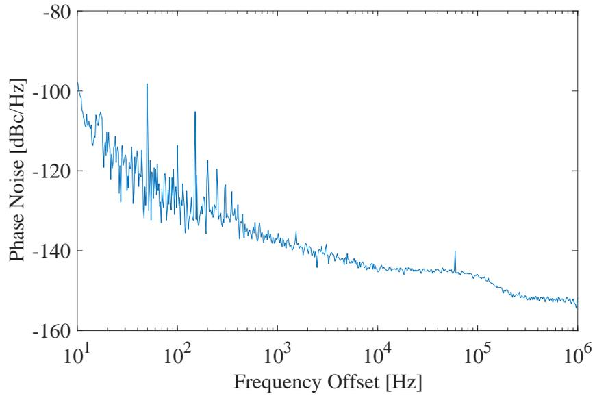
Figure 4.14: Phase noise of 81.25 MHz sampling clock. The RMS jitter from 10 Hz to 1 MHz is 114 fs.
