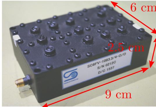
Figure 5.5: Customized 1083 MHz filter from Sogo Electronics, Inc. The designed filter bandwidth is 4 MHz.
