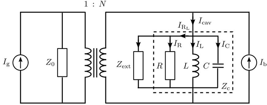
Figure 2.15: Equivalent circuit of cavity coupled to generator and beam.
