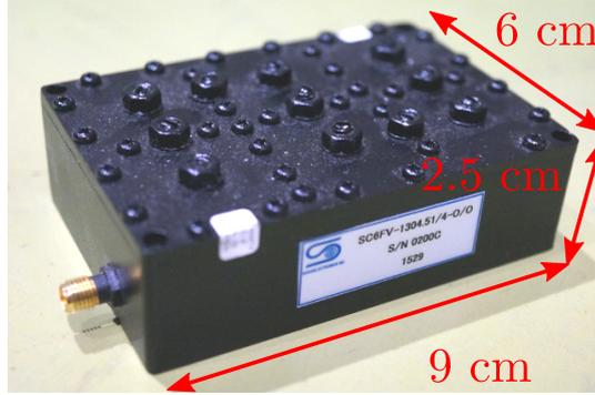
Figure 4.7: Customized 1304.5 MHz filter from Sogo Electronics, Inc. The designed filter bandwidth is 4 MHz.
