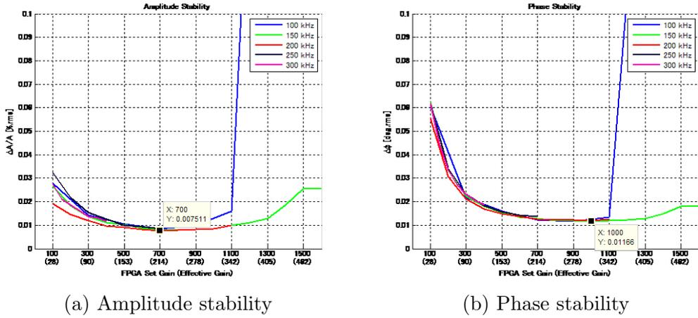
Figure 3.9: (a) Amplitude and (b) phase stability for various feedback gains and digital filter bandwidths.
