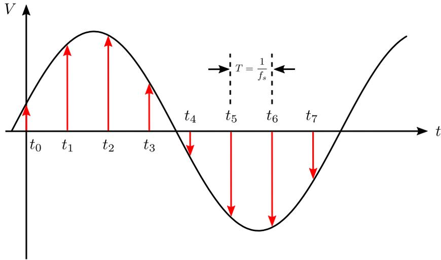
Figure 2.4: Concept of digitization of analog signal digitization. Analog signal is sampled at discrete interval with the same period  $T$ . Each sampled signal is then quantized.
