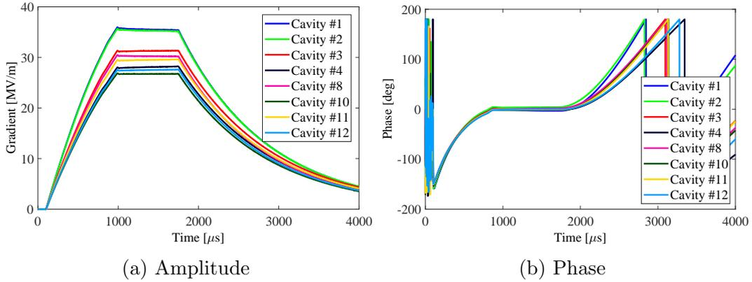
Figure 3.14: Waveform of amplitude and phase of eight cavities connected only to master board.
