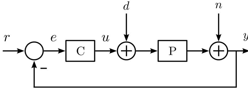
Figure 2.13: Basic closed-loop feedback control system. C is the controller, and P is the plant.
