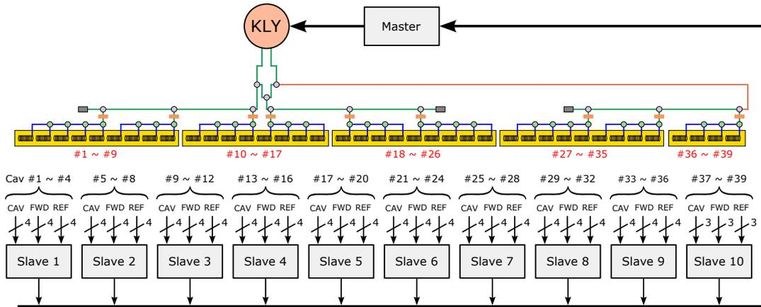
Figure 7.2: Possible configuration of digital LLRF with master–slave configuration for the ILC. Nine slave boards are required to accommodate 117 signals. CAV = cavity field; FWD = forward signal; REF = reflected signal.
