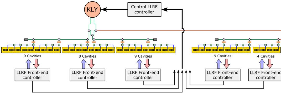
Figure 2.18: Digital LLRF control system with master–slave configuration based on the ILC TDR. LLRF front-end controller measures the signal from the cavities and sends the result to the central LLRF controller, in which the control algorithm is applied to regulate the klystron output [1].
