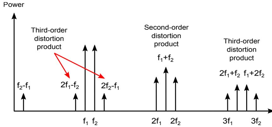
Figure 4.2: Output spectrum of nonlinear device when a two-tone input is provided.
