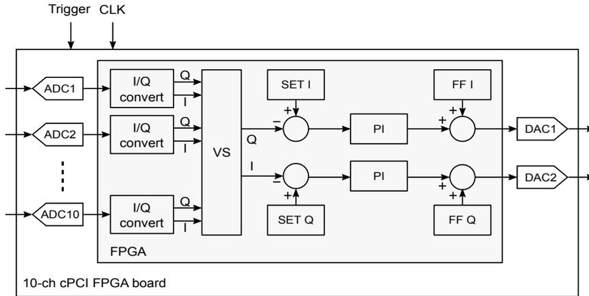
Figure 6.12: Block diagram of cPCI hardware. The board is equipped with 10 ADCs and 2 DACs.
