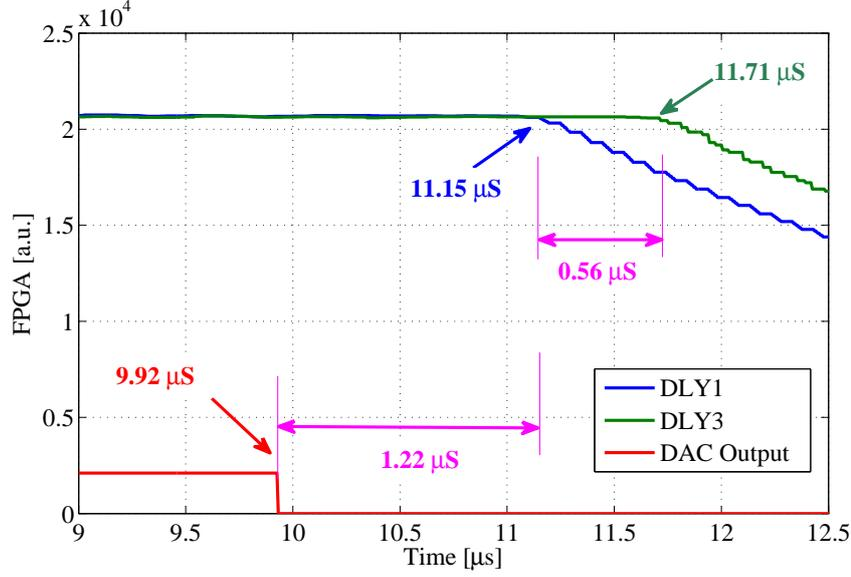
Figure 3.5: Forward signal is used to estimate the optical link communication delay and loop delay. DAC output signal is the starting point of the signal (see Figure 3.4). The signal then travels to the klystron and is finally fed to ADCs on both the slave and master boards.
