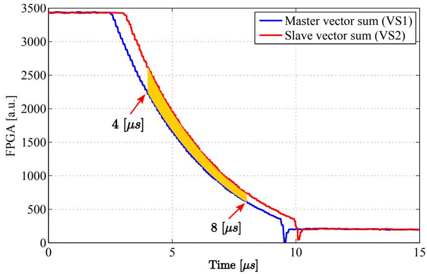
Figure 3.6: Squared area between master vector sum (VS1) and slave vector sum (VS2) was calculated from approximately 4–8  $\mu\text{s}$  for each additional delay value of VS1.
