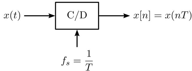
Figure 2.5: Continuous to discrete time converter block diagram.
