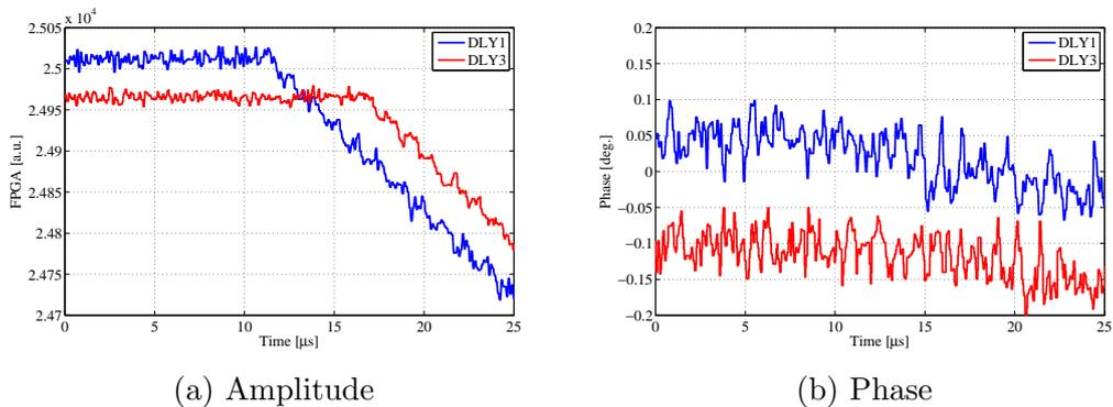
Figure 3.16: Amplitude and phase waveform at the end of Pf signal from the measurement using the setup in Figure 3.4. Additional delay of 800 clk was added to the DLY3.
