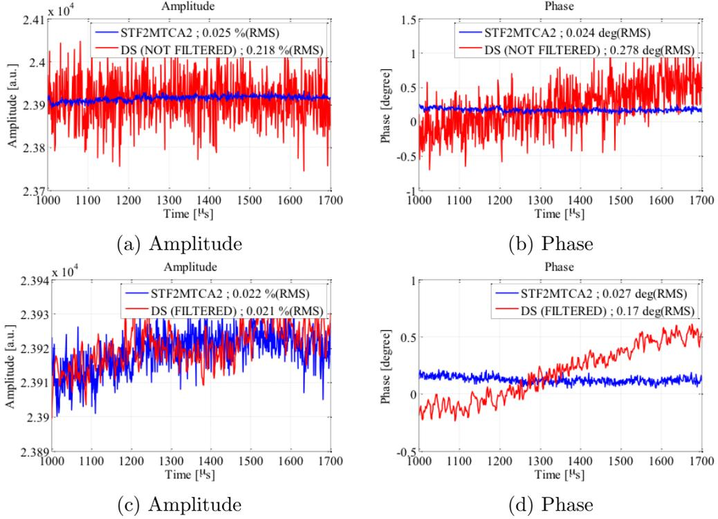
Figure 5.8: Comparison of amplitude and phase of STF2MTCA2 and direct sampling for cavity #1 with (a) and (b) the direct sampling filter off and (c) and (d) the direct sampling filter on.
