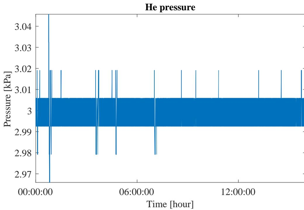
Figure 6.8: Helium pressure during 16 hours operation.
