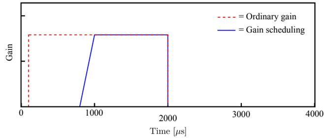
Figure 6.19: Feedback gain pattern
