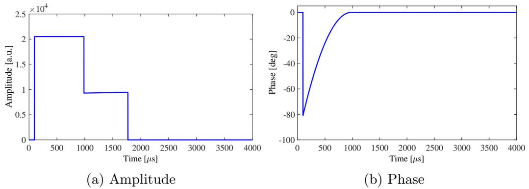
Figure 6.10: Figure (c) and (d) are the feedforward amplitude and phase table after being phase modulated. Only the phase is affected.
