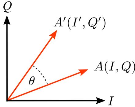
Figure 2.7: Vector  $A$  is rotated by  $\theta$
