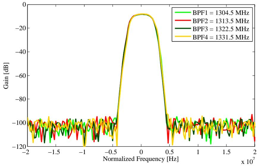
Figure 4.10: Frequency response of two cascaded filter. The filter frequencies are normalized.
