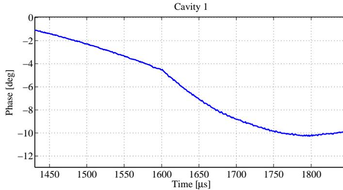
Figure 6.2: The example of phase decay after the RF power is turned off at 1600  $\mu\text{s}$
