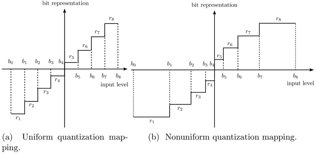
Figure 2.6: Quantization mapping diagram. An input level  $b_k$  is mapped to bit representation  $r_k$ .
