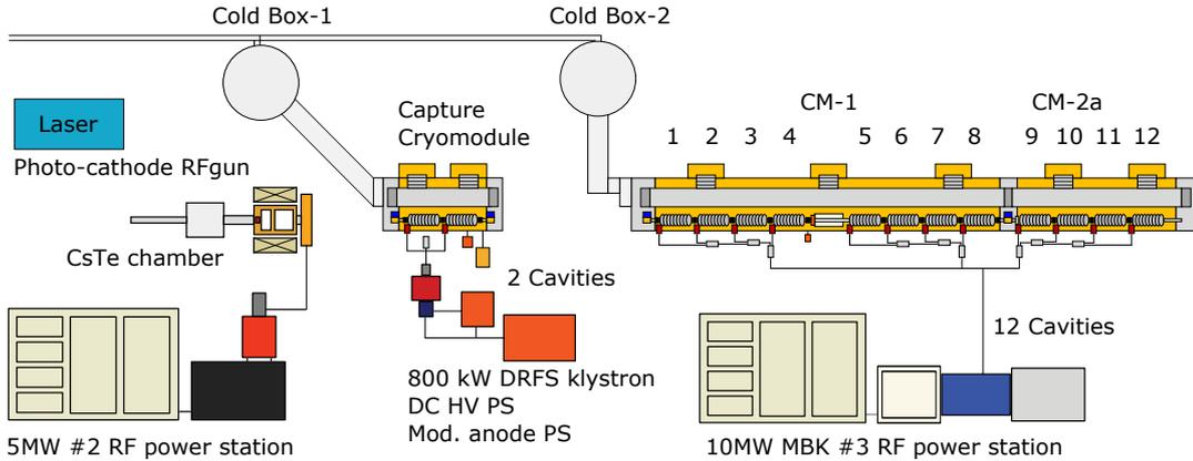
Figure 1.4: Layout of the STF. It consists of a normal conducting photo-cathode RF gun, two superconducting nine-cell cavities in the capture cryomodule, eight superconducting nine-cell cavities in the cryomodule CM-1, and four superconducting nine-cell cavities in the cryomodules CM-2a.
