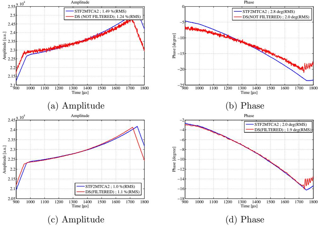
Figure 5.9: Comparison of amplitude and phase of STF2MTCA2 and direct sampling for cavity #8 with (a) and (b) the direct sampling filter off and (c) and (d) the direct sampling filter on.
