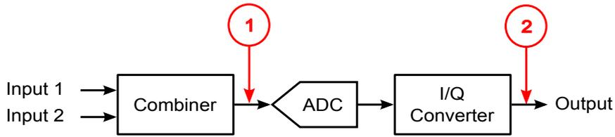
Figure 4.3: Two-tone measurement setup. Test point 1 is the output of the combiner and is measured by a spectrum analyzer. Test point 2 is the output of the I/Q converter and is estimated using Equations 2.7 and 2.8. The magnitude of the I/Q converter output is changed to dBFS.
