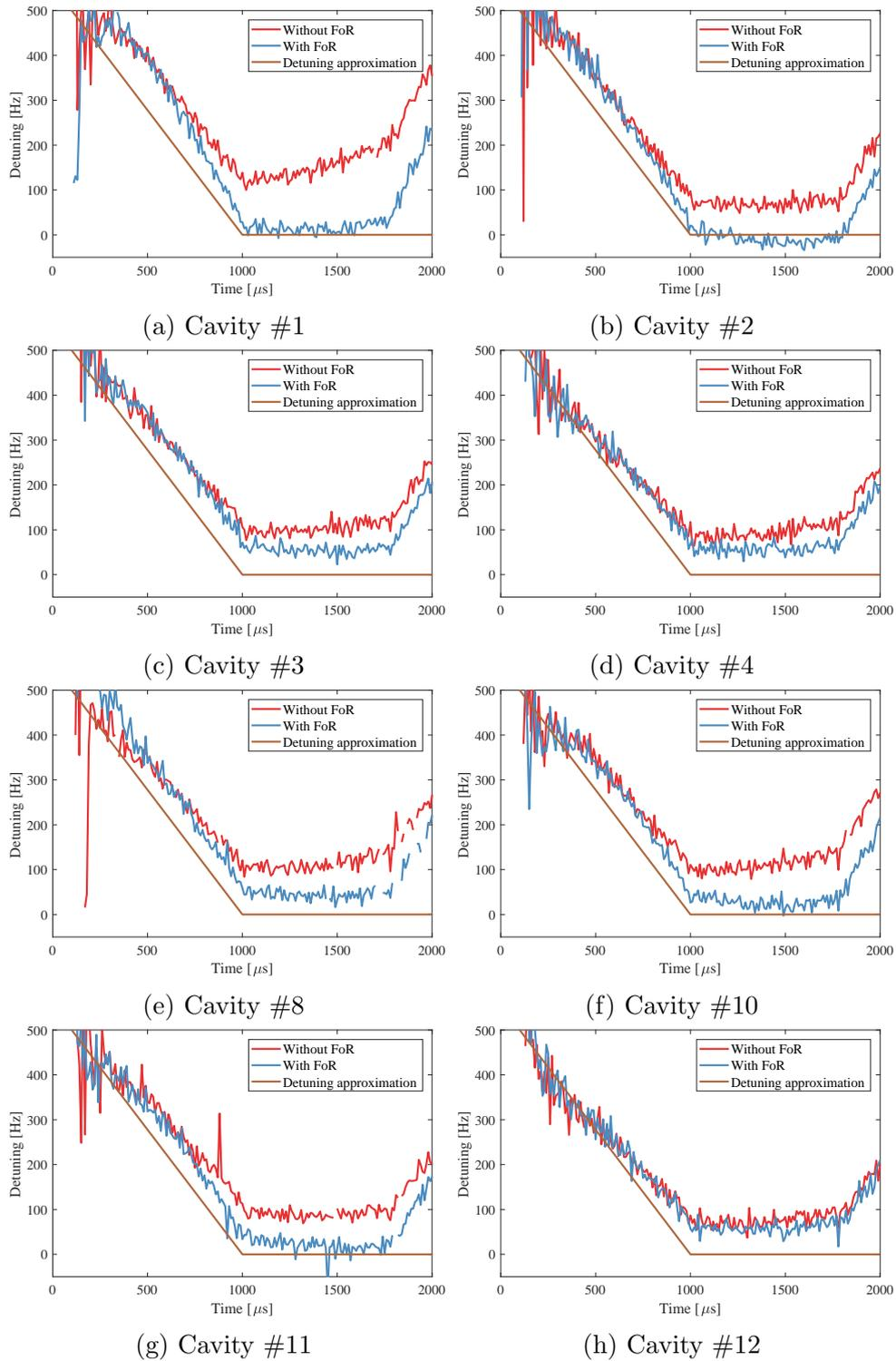
Figure 6.17: Detuning patterns of all cavities without and with filling on resonance (FoR).
