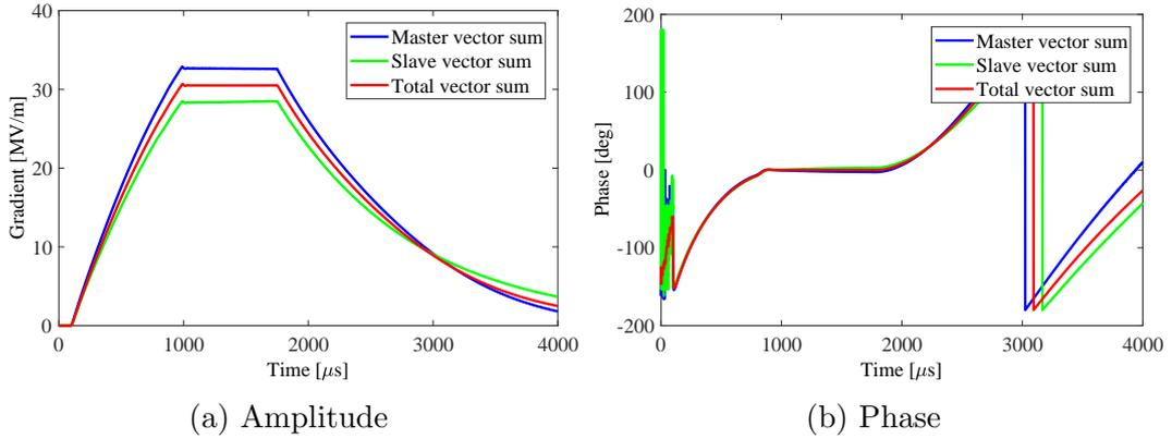
Figure 3.12: Amplitude and phase of partial vector sum from slave and master and total vector sum. The average flattop gradient are *Master vector sum* (VS1) = 32.6 MV/m, *Slave vector sum* (VS2) = 28.4 MV/m, and *Total vector sum* = 30.5 MV/m
