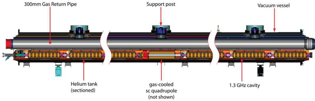
Figure 1.3: Type B cryomodule consists of eight cavities and a quadrupole in the middle. In the type A cryomodule, the superconducting cavity is installed instead of the quadrupole. [1]
