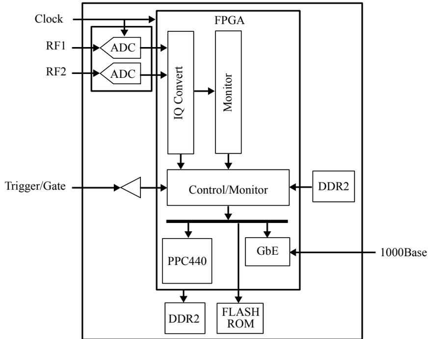
Figure 5.7: Block diagram of MTCA.0-compliant board for direct sampling.
