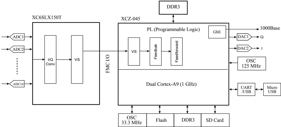
Figure 3.3: Schematic of the MTCA.4-compliant front. It is composed of two FPGAs: a Spartan 6 (XC6SLX150T) and a Xilinx Zynq-7000 (XCZ045).
