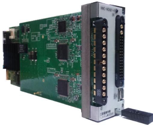
Figure 5.6: MTCA.0-compliant digital LLRF board for direct sampling.
