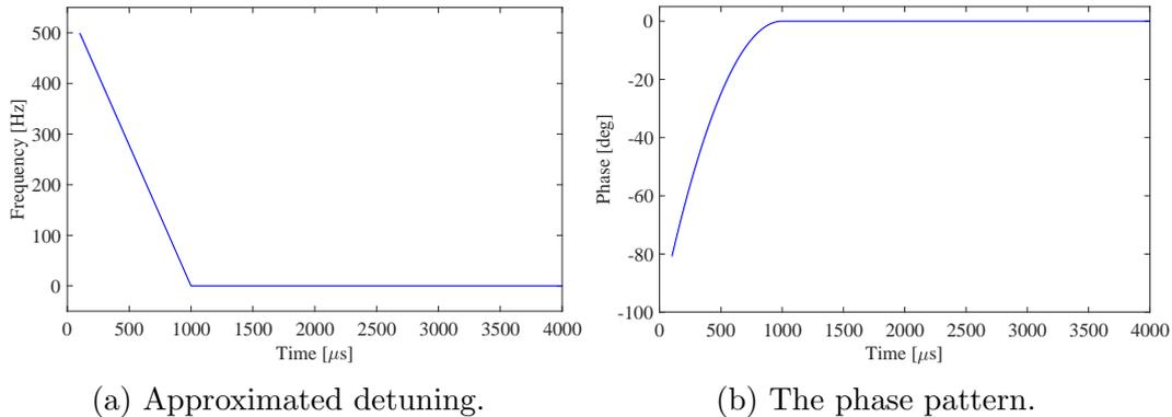
Figure 6.9: The upper figure is the detuning pattern approximated from a simple linear fitting. Right figure is the phase pattern calculated from approximated detuning using equation 6.2.
