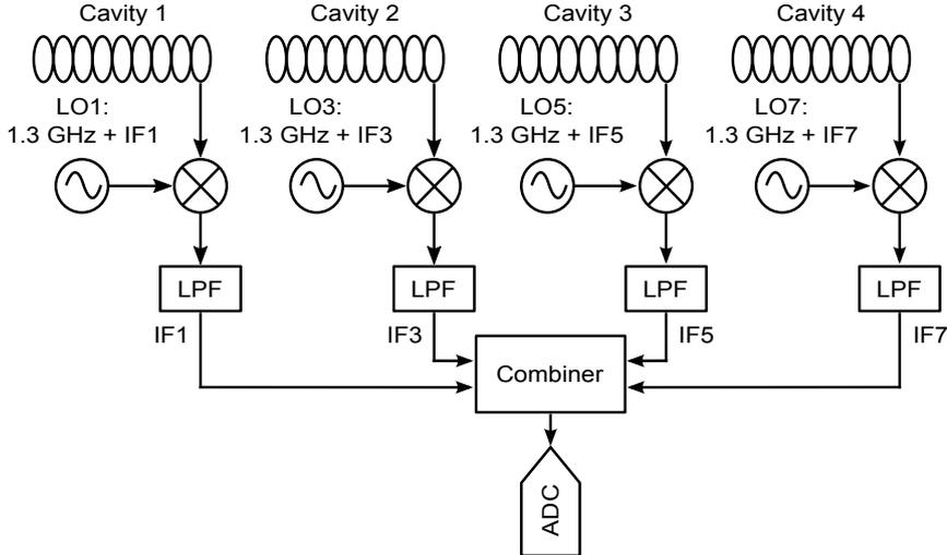
Figure 4.1: Front-end for multi-IF Technique. Each cavity output is mixed with a different LO frequency and filtered by an LPF with the corresponding frequency. Four IFs are combined by a passive power combiner, and its output is connected to one ADC.
