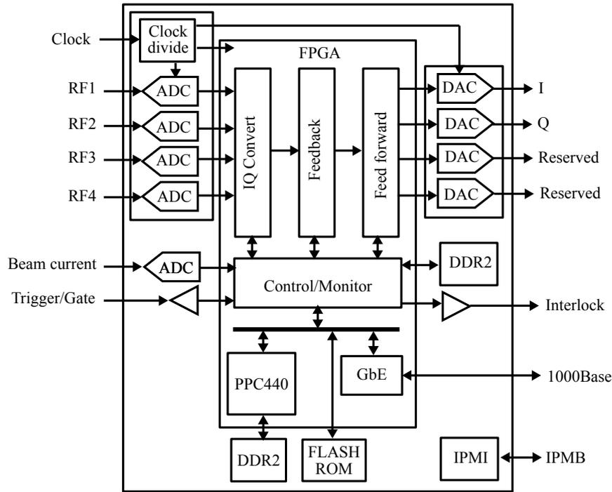
Figure 4.13: Block diagram of digital LLRF board with MTCA.0 configuration. The board is equipped with four ADCs and four DACs.
