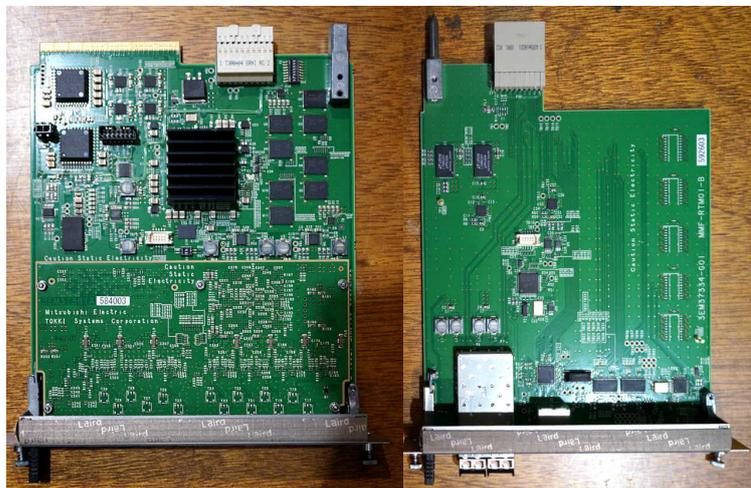
Figure 3.2: MTCA.4-compliant board for master–slave configuration. Left: front board equipped with 14 ADCs (AD9650), 2 DACs (AD9783), and Xilinx Zynq-7000 and Spartan 6 FPGAs. Right:  $\mu$ RTM (MTCA Rear Transition Module) equipped with a gigabit ethernet card (RJ-45), small form-factor plugable connector, and digital input/output.
