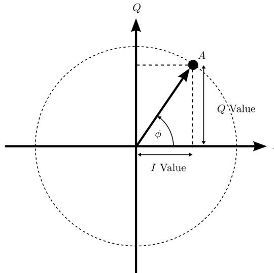
Figure 2.3: Representation of signal in the Cartesian coordinates. The symbol of  $A$  and  $\phi$  are the amplitude and phase, respectively. The  $I$  component is the in-phase or real part and the  $Q$  component is the quadrature or imaginary part.
