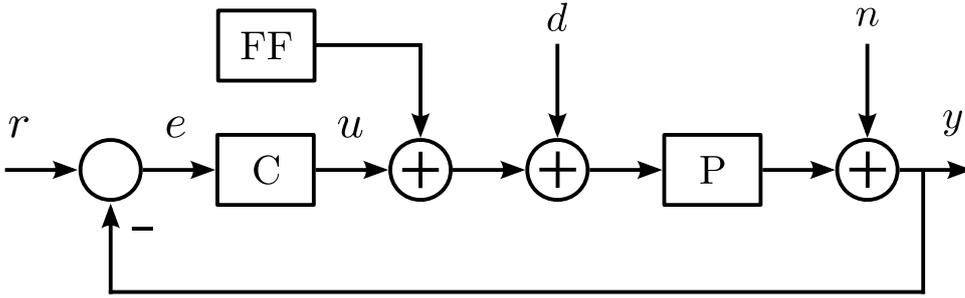
Figure 2.14: Proportional and feedforward control system. FF is feedforward controller, C is proportional controller. and P is the plant.
