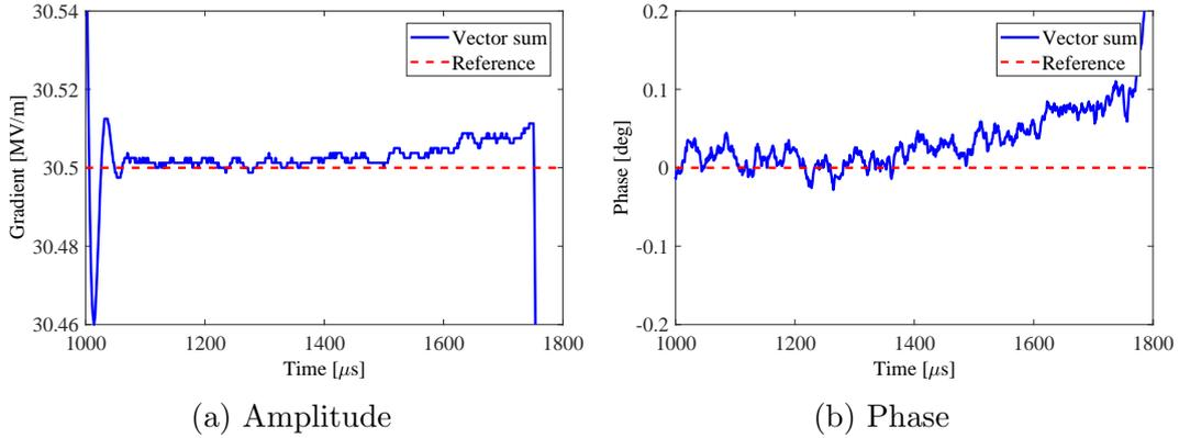
Figure 3.15: Flattop of vector sum of eight cavities operated with only master board.
