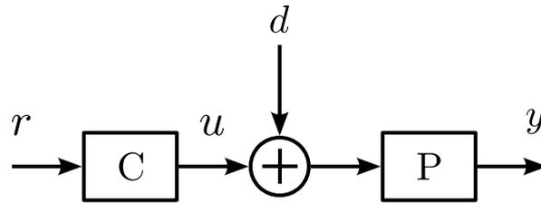
Figure 2.12: Open-loop control system. C is the controller, and P is the plant.
