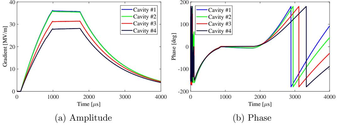
Figure 3.10: Amplitude and phase of cavities #1, #2, #3, and #4. The mean flattop gradients of each cavity are 35.8 MV/m (cavity #1), 35.6 MV/m (cavity #2), 31.3 MV/m (cavity #3), and 28.0 MV/m (cavity #4).
