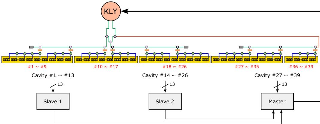
Figure 7.1: Possible configuration of digital LLRF with master–slave configuration for the ILC. Using three boards, 39 signals can be accommodated. However, in this configuration, only cavity field signals can be measured
