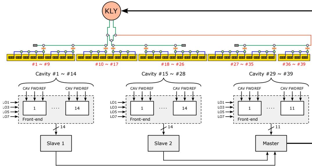
Figure 7.3: Possible digital LLRF control system for the ILC using master-slave configuration and four IFs. The front-end block is illustrated in detail in Figure 4.1. CAV = cavity field; FWD = forward signal; REF = reflected signal.
