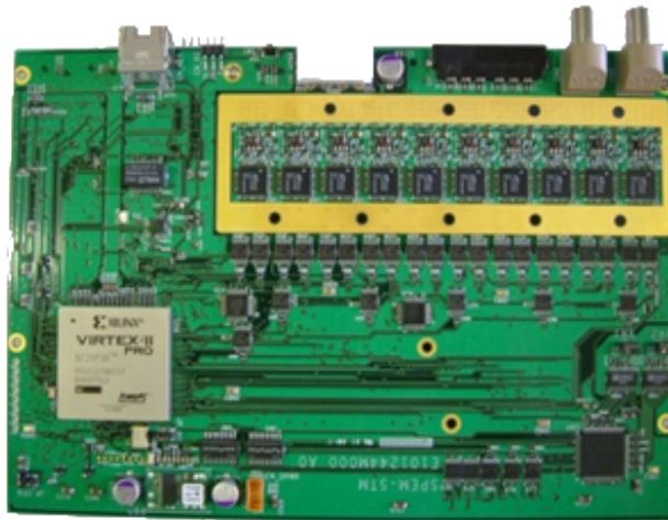
Figure 6.11: cPCI-compliant digital LLRF board.
