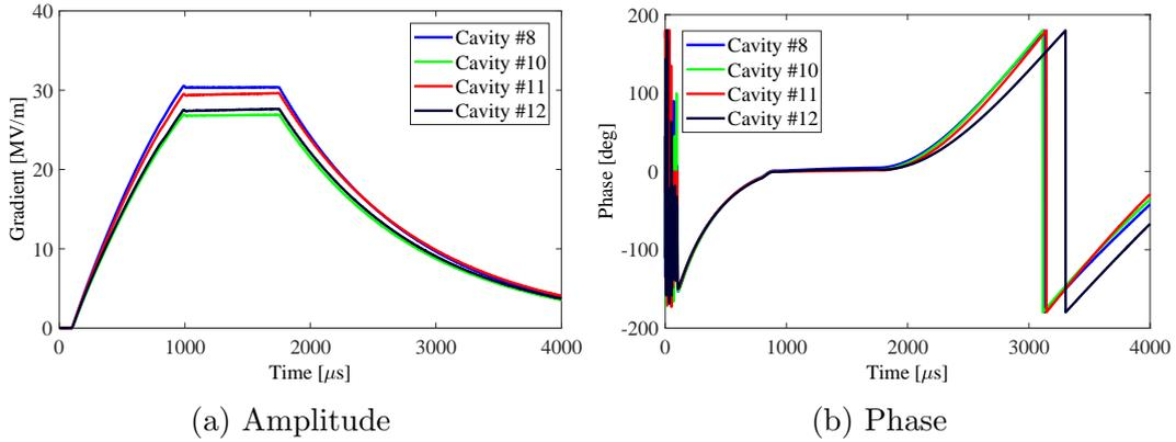
Figure 3.11: Amplitude and phase of cavities #8, #10, #11, and #12. The average flattop gradients of each cavity are 30.3 MV/m (cavity #8), 26.8 MV/m (cavity #10), 29.5 MV/m (cavity #11), and 27.5 MV/m (cavity #12).
