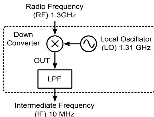
Figure 2.2: Simplified down conversion schematic. The process is actually multiplication of two inputs. The multiplication yields two frequencies, but only one frequency (the IF) is extracted by filtering the other frequency out.
