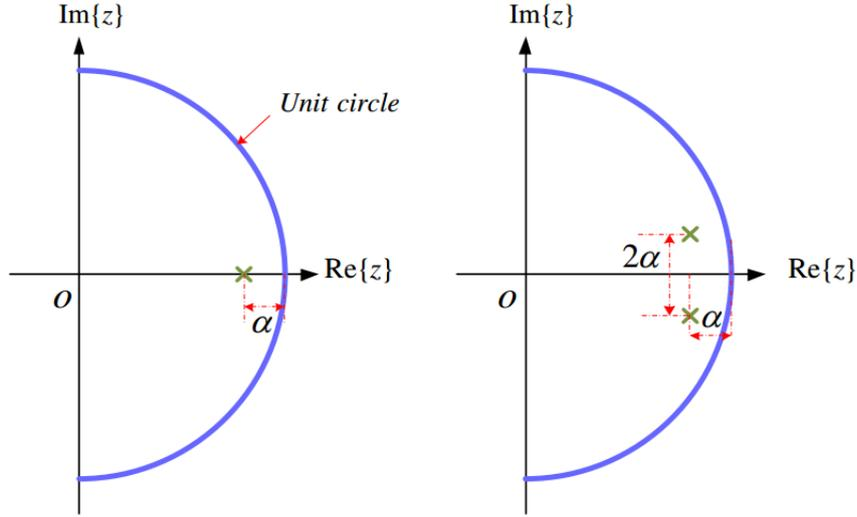
Figure 2.10: Poles-zero plot of first order digital IIR filter (left) and conjugate pole filter (right) [14].
