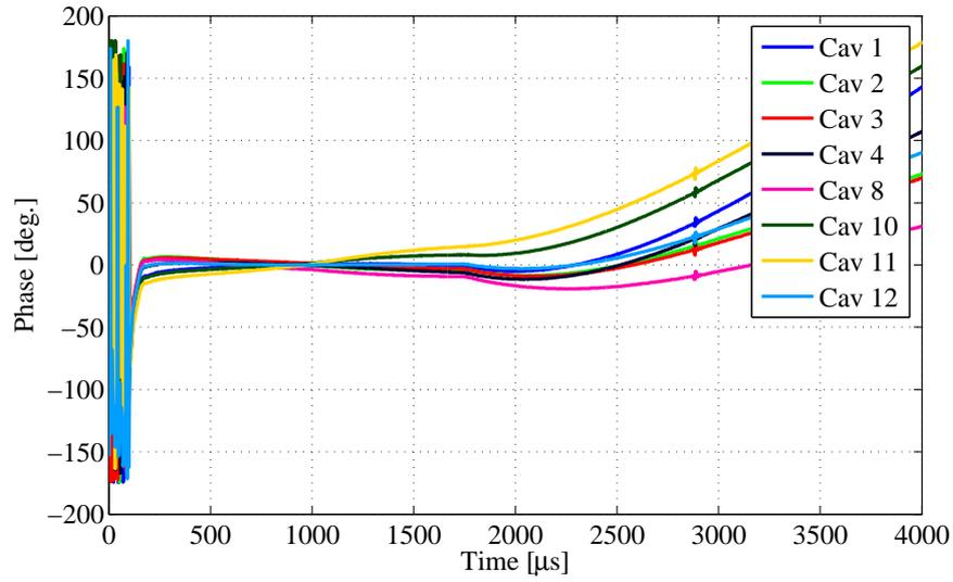
Figure 4.16: Phase waveform of eight cavities.
