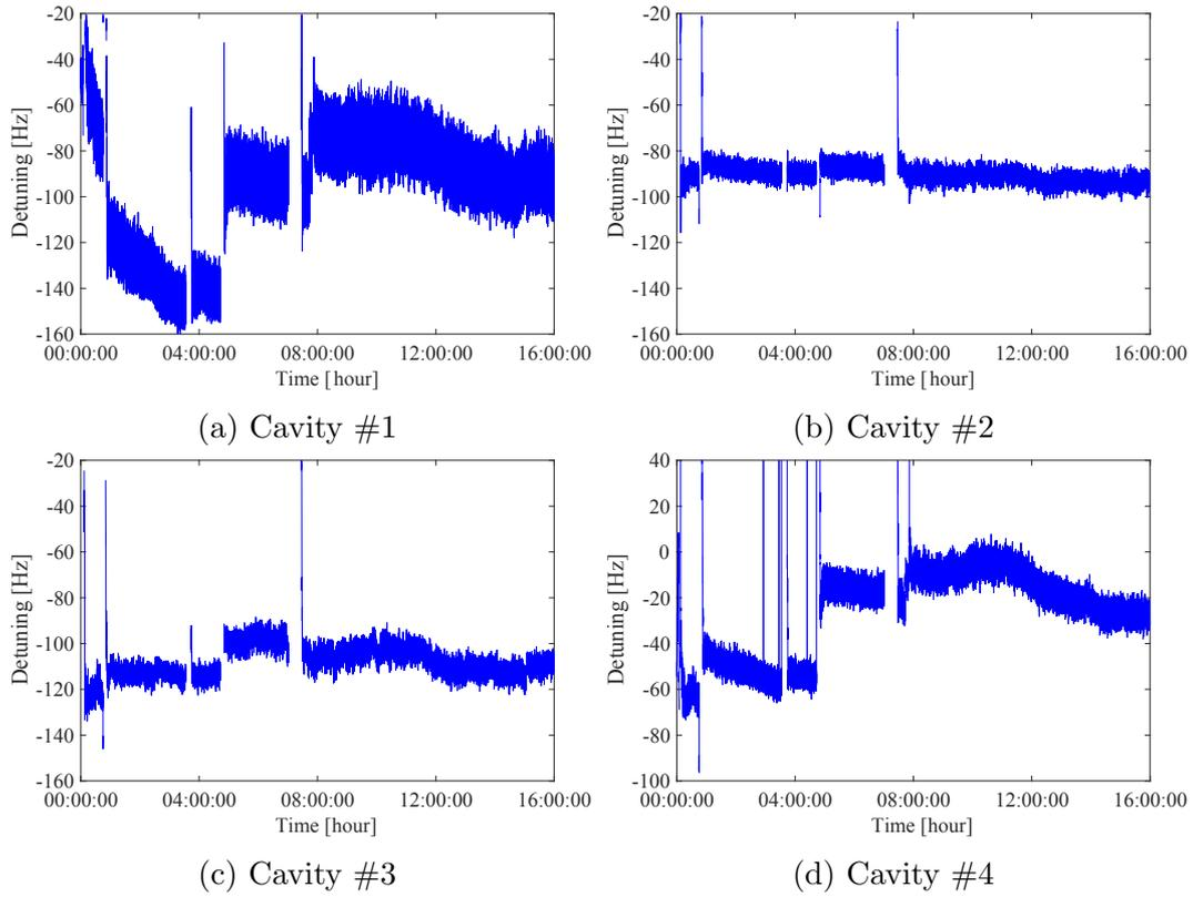
Figure 6.6: Detuning of cavities #1, #2, #3, and #4 at the end of the RF pulse. Data were taken for 16 h, as indicated on the time axis of the detuning plot.
