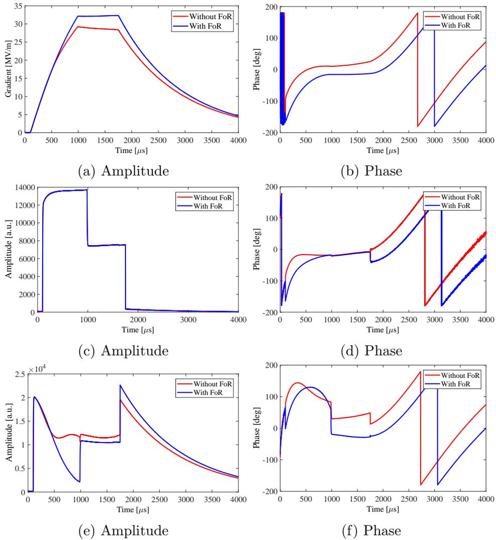
Figure 6.13: Forward, cavity pickup, and reflected waveforms without and with filling on resonance method.
