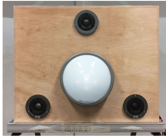
Figure 5.10. Transmitter for ToA localization using VLC synchronization.
