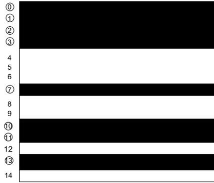
**Figure 3.8:** A simple one-dimensional optimum-coded mask based on the modulo 15 cyclic difference set (0, 1, 2, 3, 7, 10, 11, 13). This figure is adapted from Ref. [35].
