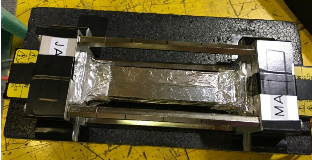
Fig.3.14. Detector system used in measurement of response to heavy charged particles.
