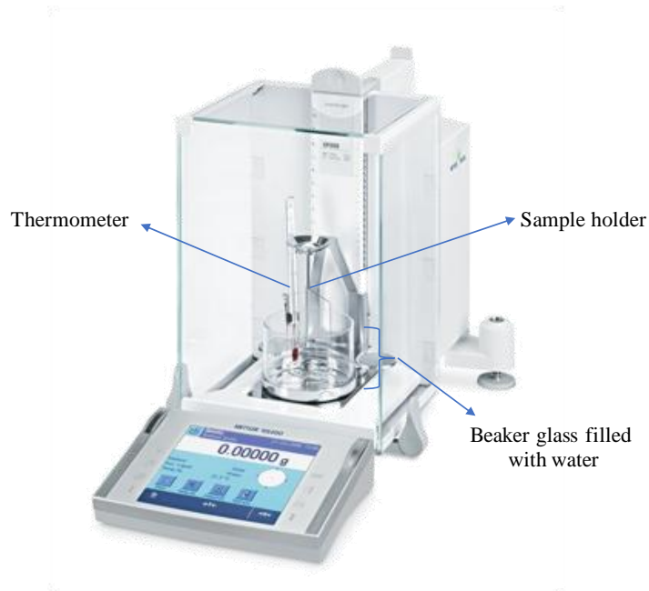
Figure 5. 7 The density determination kit of METTLER TOLEDO balance. [116]
