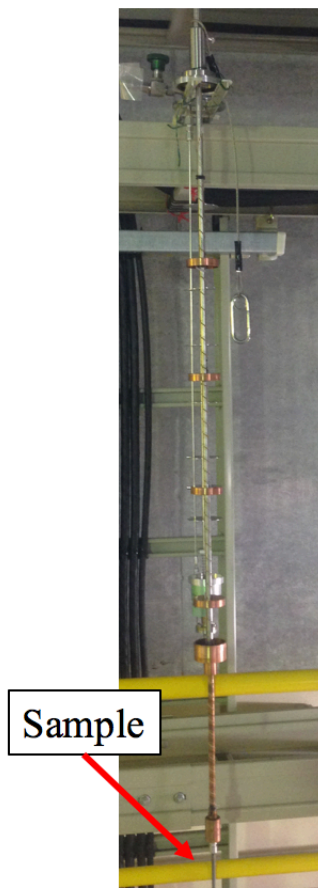
Fig. 2.5.5. Pictures of (a) sample rod and (b) refrigerator of magnet option.
