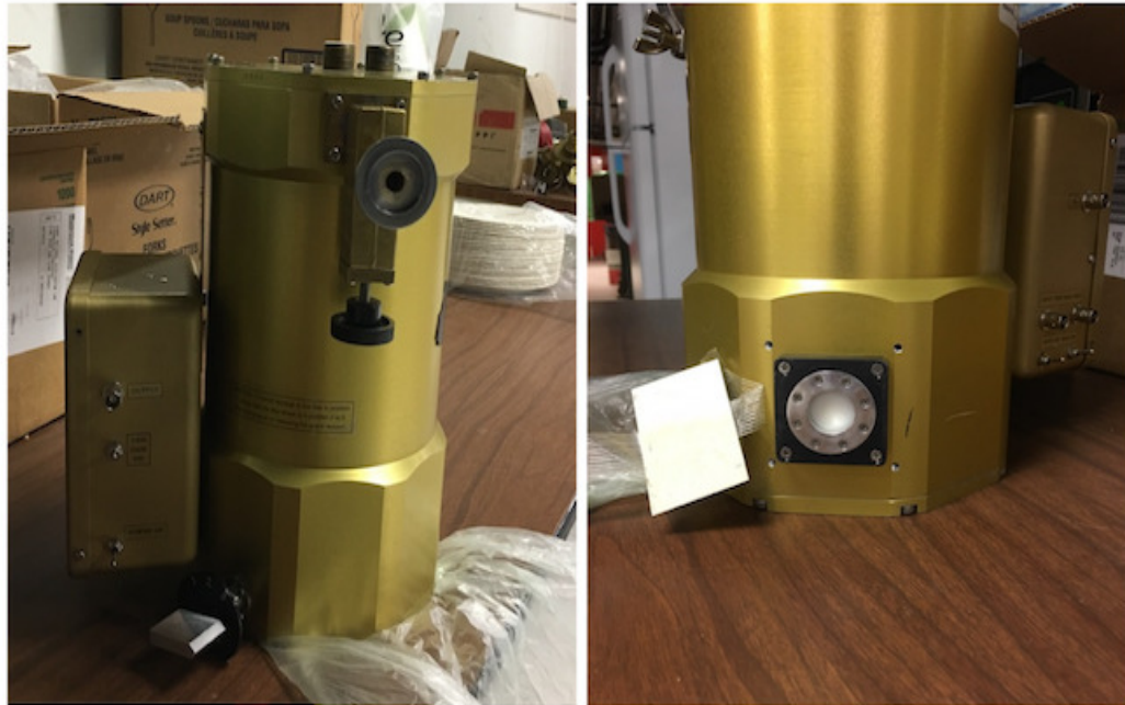
FIGURE 7.20: A He-cooled bolometer (HDL-5 model, IRLabs). The left picture represents a window of the bolometer.
