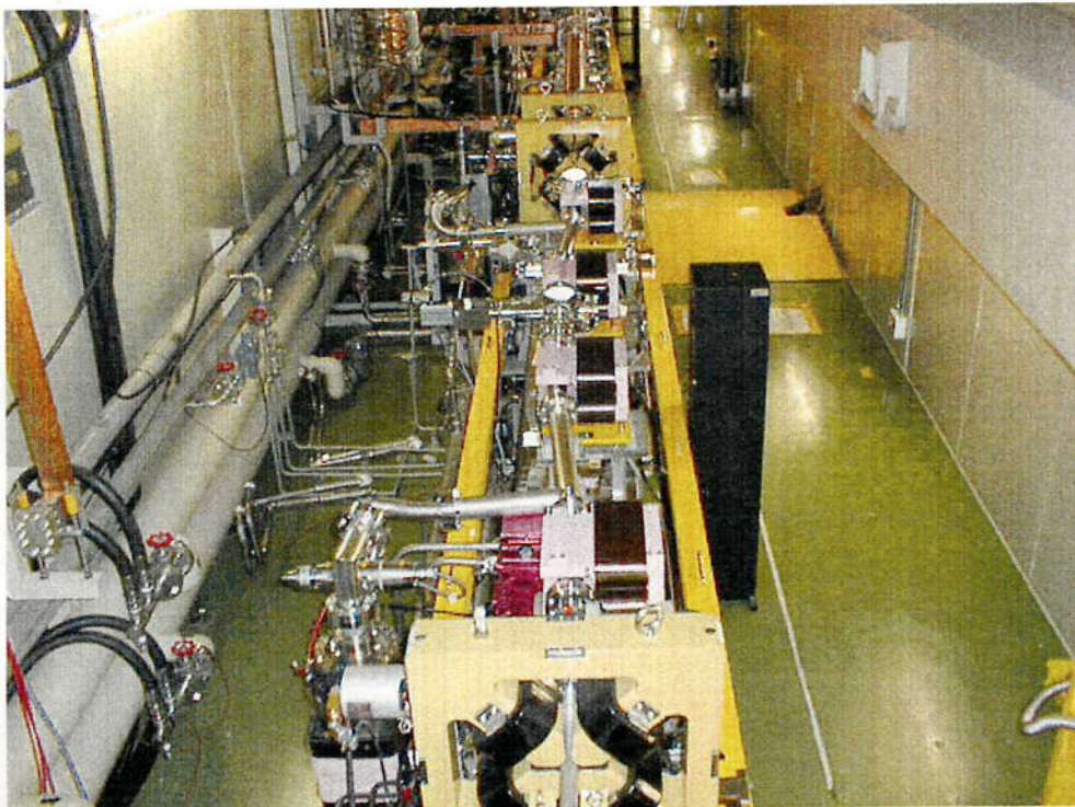
Figure 4.19: Photograph of the chicane to measure the multi-bunch beam energy at the middle of linac. The chicane was constructed by four dipole magnets and it contains a beam position monitor and beam profile monitor.
