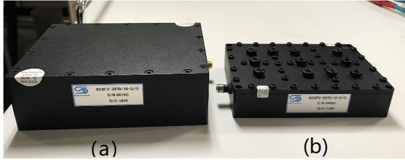
Figure 5.4: BPFs used in the monitoring system. (a) Customized waterproof type BPF to reduce the monitoring system phase drift, (b) normal cavity-type BPF, initially used in the monitoring system.
