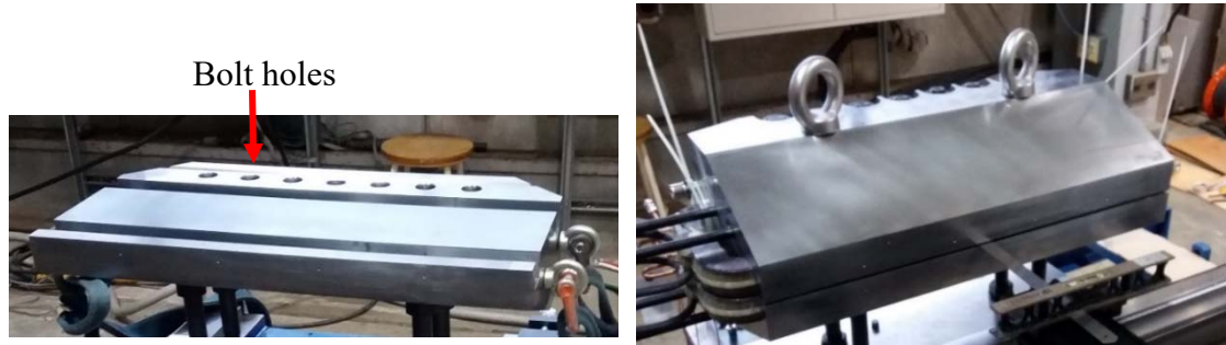
Figure 7.4: Lower part of the iron core (left) and assembled iron core (right).
