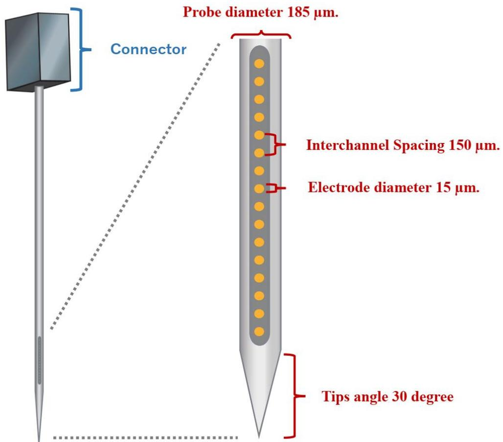
**Figure 4: Schematic representation of the multi-channel electrode. This electrode was used to record pallidal activity during task performance. The electrode had 16 contacts linearly arranged with 150  $\mu\text{m}$  inter-channel spacing. (Electrode diameter = 15  $\mu\text{m}$ , Probe diameter = 185  $\mu\text{m}$ , Impedance  $275 \pm 50 \text{ k}\Omega$ , distance from tip to the first channel = 500  $\mu\text{m}$ , tip angle = 30 degree).**
