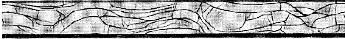
Fig. 7.4.5-3: Unfolded images of ferrite echoes from ferrite surface and ferrite/copper boundary. Horizontal and vertical directions correspond to azimuthal and axial direction, respectively. Dark bands at the top and bottom of each figure correspond to tapers. This absorber (#6S3) was used for beam tests in TRISTAN AR. Cracks are clearly seen in the boundary echo as black lines. Since the widths of cracks were less than 10\ \mu\text{m} they could not be seen with surface echo (upper image). The vertical lines are not defects but the borderlines of images (the whole image consists of nine 40-degree wide images).
