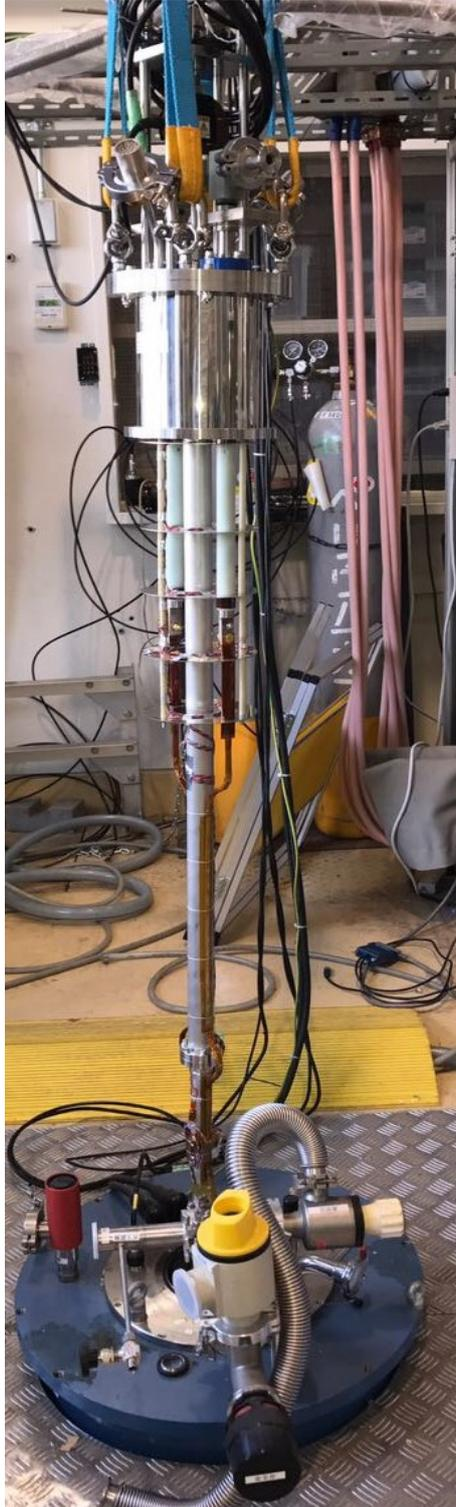
**Figure C.5:** 4.2 K test probe
