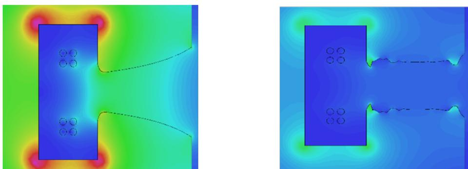
**Figure 5.1:** Convergence of pole profile from combined function (curved) to dipole (flat)
