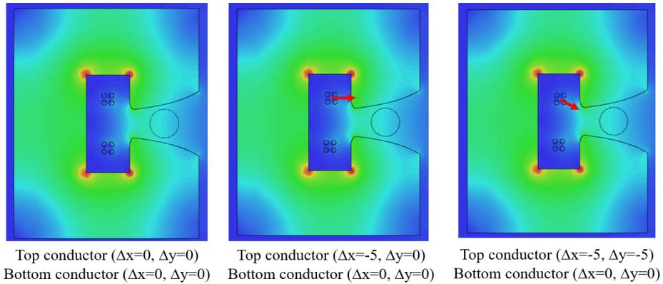
**Figure 3.10:** Movement of conductor in x and y direction
