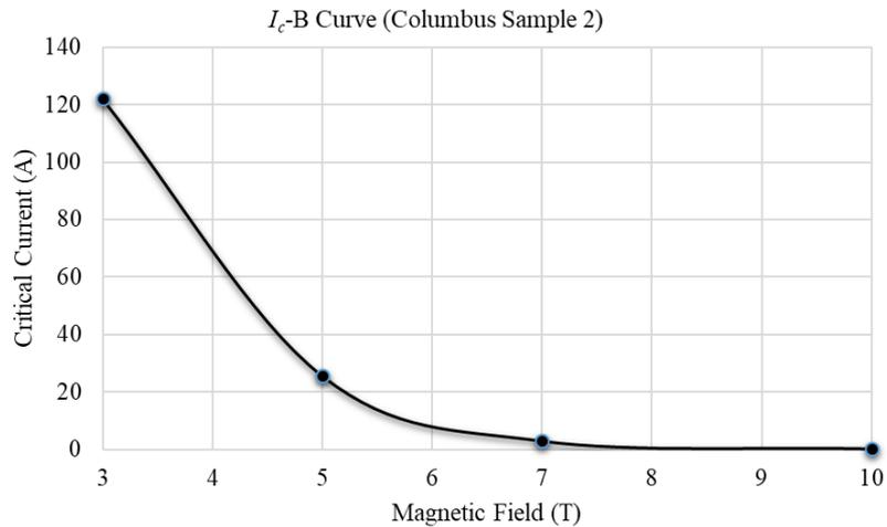
**Figure D.7:** Columbus sample 2- critical current as a function of external magnetic field
