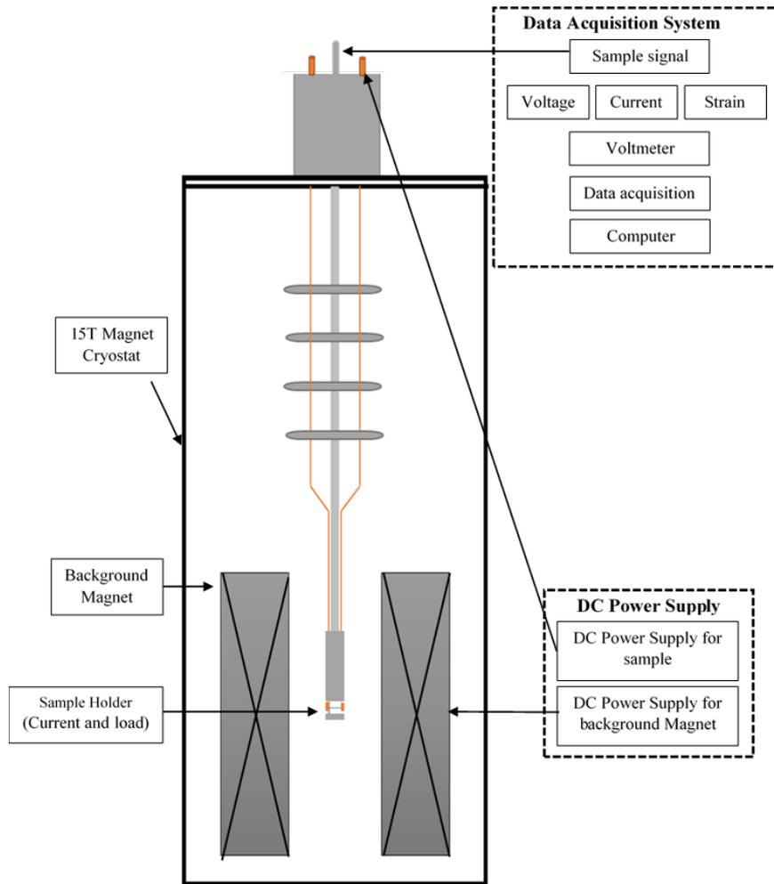
**Figure 4.13:** 4.2 K test setup
