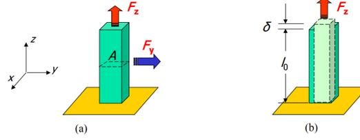
**Figure 4.1:** (a) Normal and shear stresses (b) Strain
