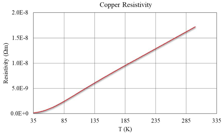
**Figure B.6:** Variation of resistivity of copper with temperature. [14]
