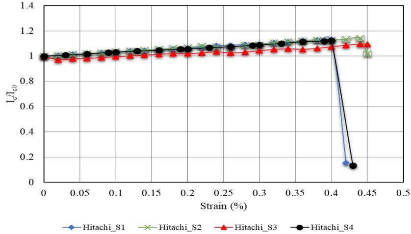
**Figure 4.18:**  $I_c/I_{c0}$  dependence on strain at 4.2 K under external magnetic field.
