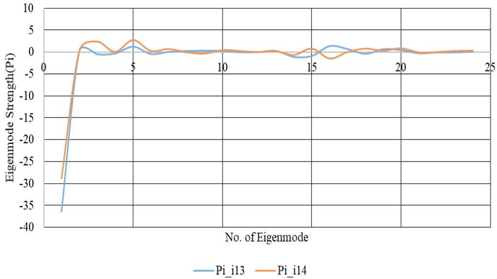
**Figure A.4:** Reduction in strength of higher eigenmodes after several iteration
