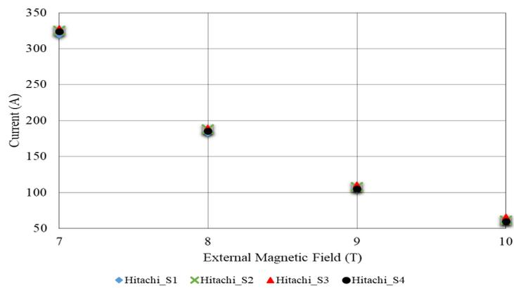
**Figure 4.15:**  $I_c$  as a function magnetic field for Hitach  $MgB_2$  wire at 4.2 K
