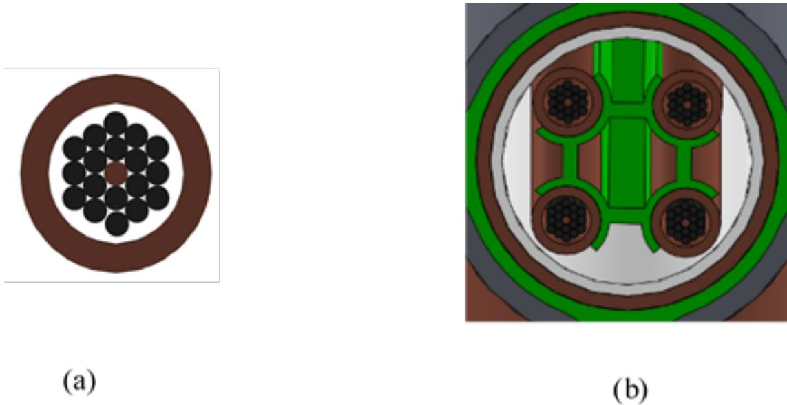
**Figure 2.4:** Proposed cable assembly for SC Transmission Line (a) Sub-unit of 20 kA cable, (b) 80 kA transmission line
