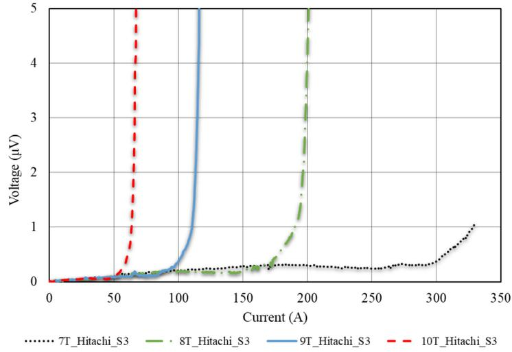
**Figure D.4:** Hitachi Sample 3 - I-V curve under variable field (7 T - 10 T) under 0 % strain
