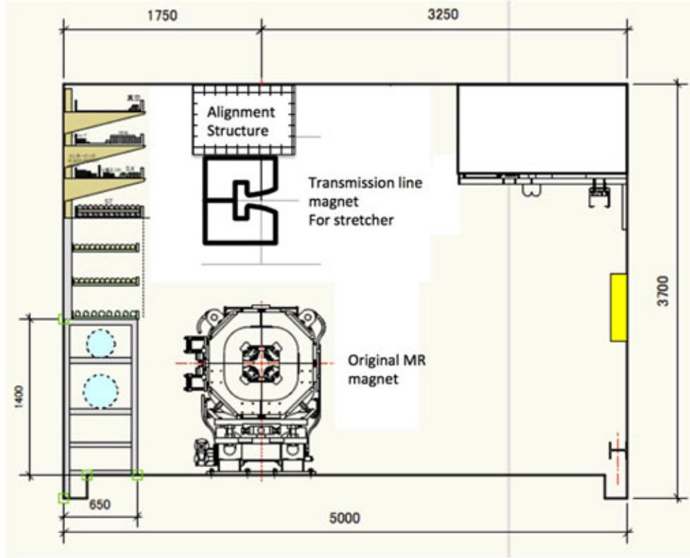
Figure 2.1: J-PARC tunnel cross section with transmission line magnet for SR
