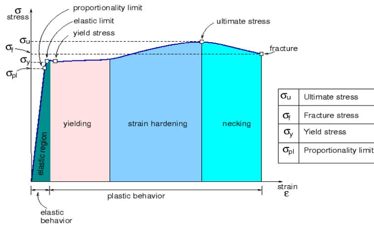
**Figure 4.2:** Stress-strain graph for a typical material
