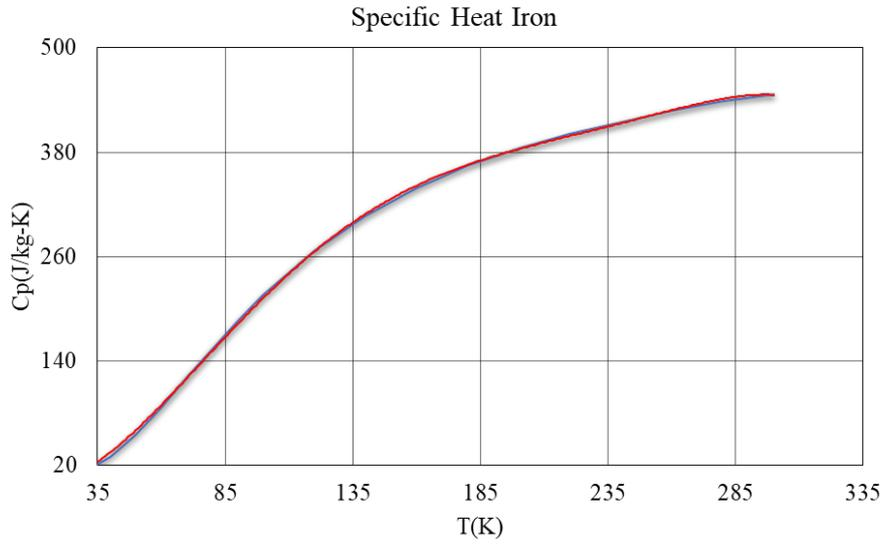
**Figure B.3:** Variation of specific heat of iron with temperature. [16]
