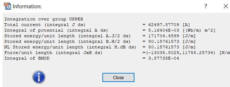
**Figure 4.3:** Total current and forces acting of transmission line [10].
