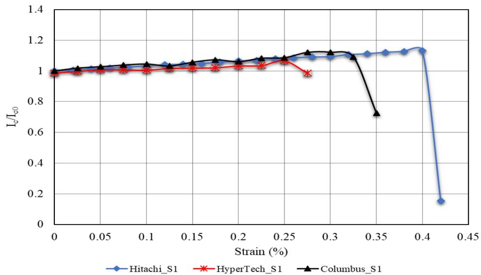
**Figure 5.3:** Comparison of  $I_c/I_{c0}$  as a function of applied strain in three  $MgB_2$  wire with different composition
