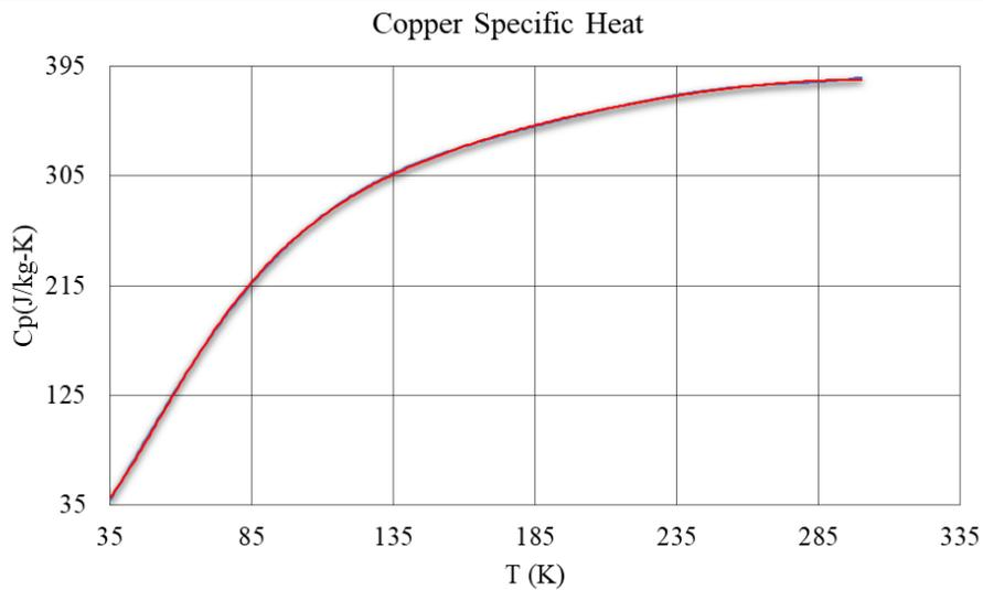
**Figure B.2:** Variation of specific heat of copper with temperature. [14]
