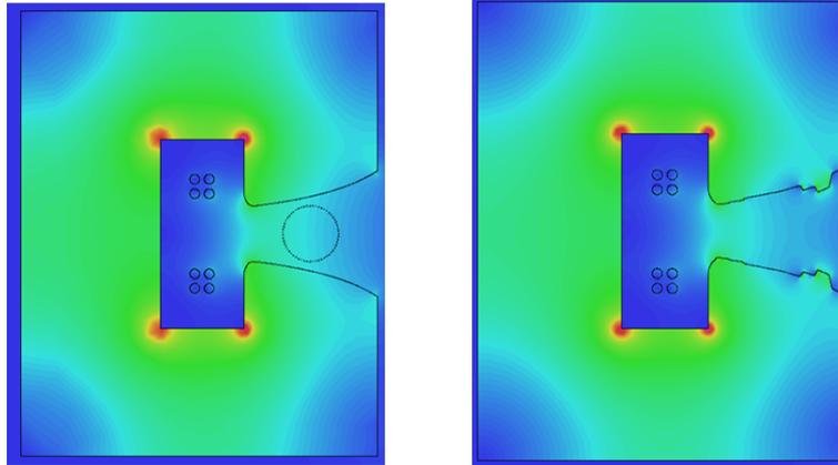
**Figure 3.6:** Pole shape shimming after improved iterative process
