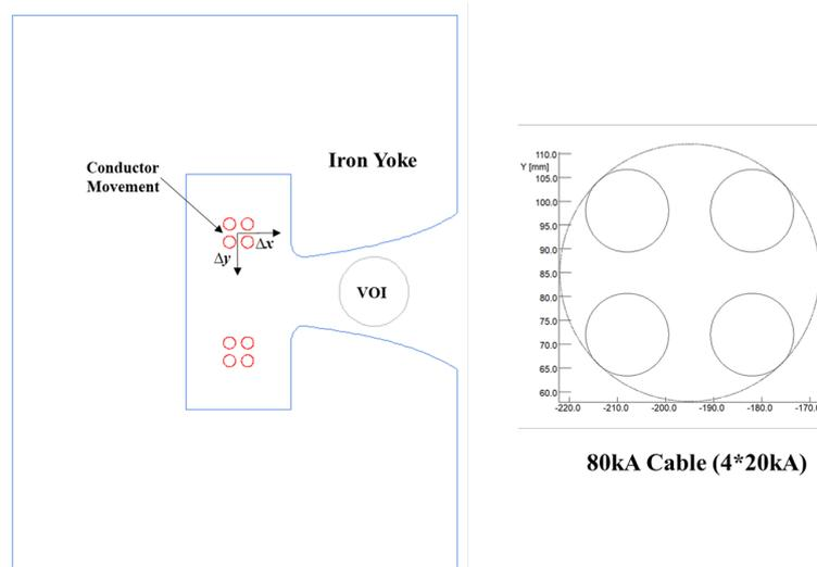
**Figure 3.9:** Schematics of iron yoke with transmission line conductor and displacement direction of conductor
