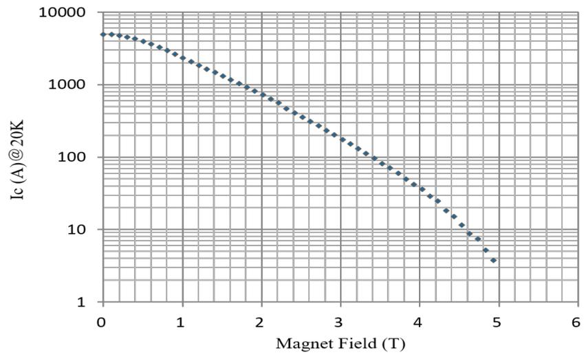
**Figure 4.20:** Critical current at 20 K under variable external field [Hitachi data]
