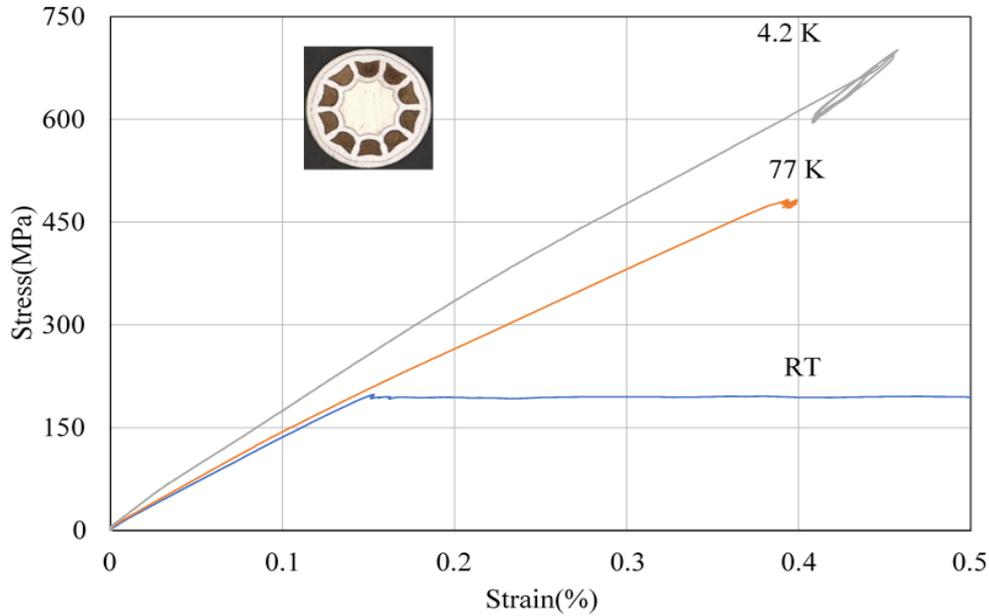
**Figure 4.12:** Stress-strain curve at variable temperature
