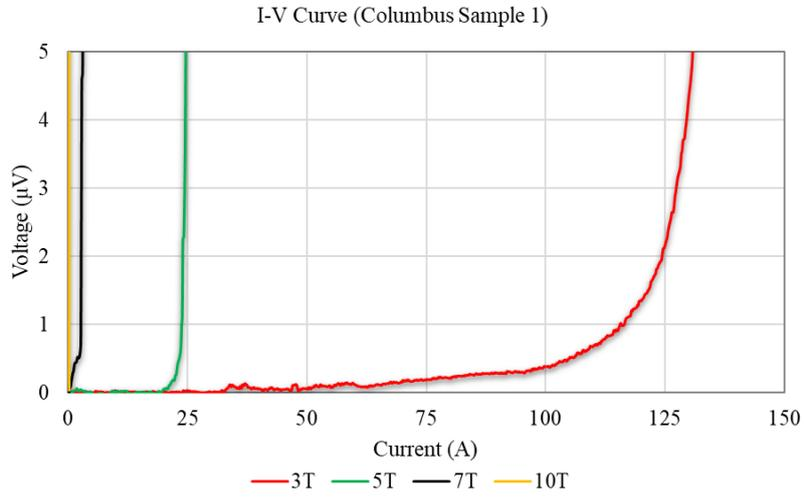
**Figure D.8:** Columbus sample 1 - I-V curve under variable field (3 T - 10 T) under 0 % strain
