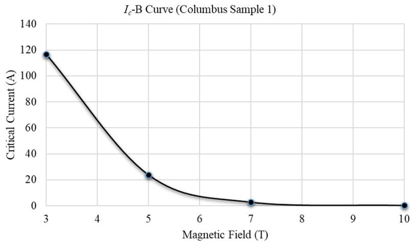
**Figure D.6:** Columbus sample 1- critical current as a function of external magnetic field
