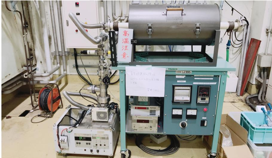
**Figure C.1:** Vacuum furnace for annealing sample wire
