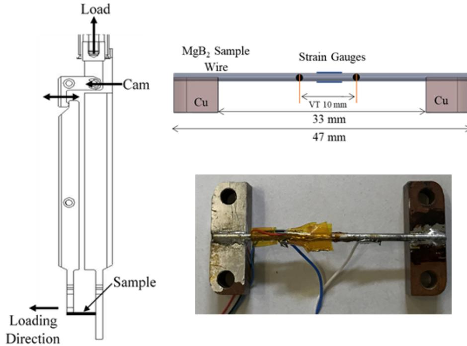
**Figure 4.14:** Schematic of direction of applied load and investigating sample
