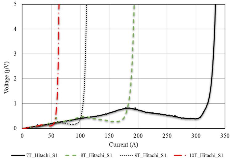
**Figure D.2:** Hitachi Sample 1 - I-V curve under variable field (7 T - 10 T) under 0 % strain
