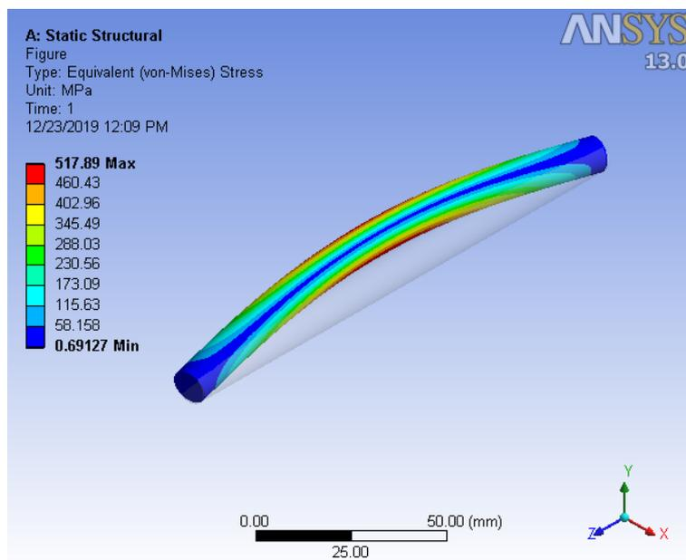
**Figure 4.7:** Stress distribution in 150 mm length cable.
