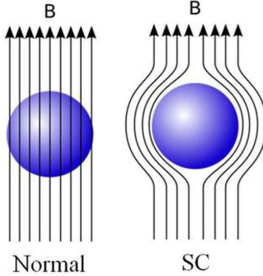
**Figure 1.2:** meissner effect, normal and superconductor
