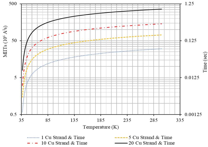
**Figure 4.21:** MIITs and time dependence of temperature based on the copper ratio in  $\text{MgB}_2$  cable
