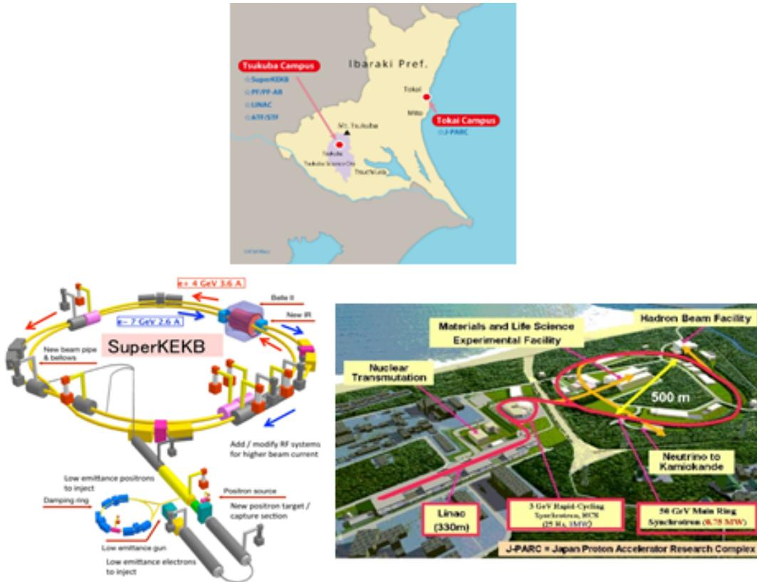
**Figure 1.8:** KEK and J-PARC accelerator complex layout
