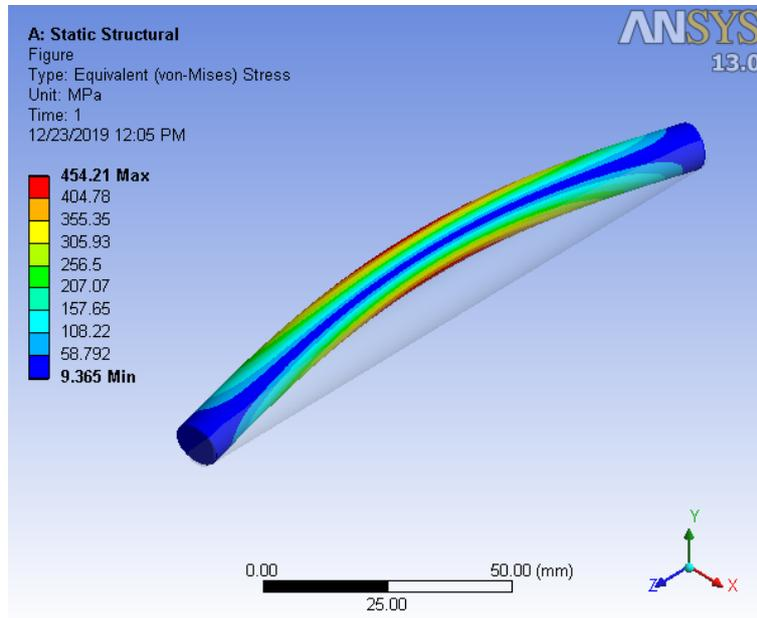
**Figure 4.6:** Stress distribution in 140 mm length cable.
