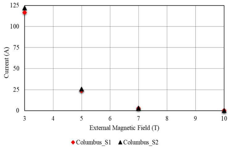
**Figure 4.17:**  $I_c$  as a function magnetic field for Columbus  $MgB_2$  wire at 4.2 K
