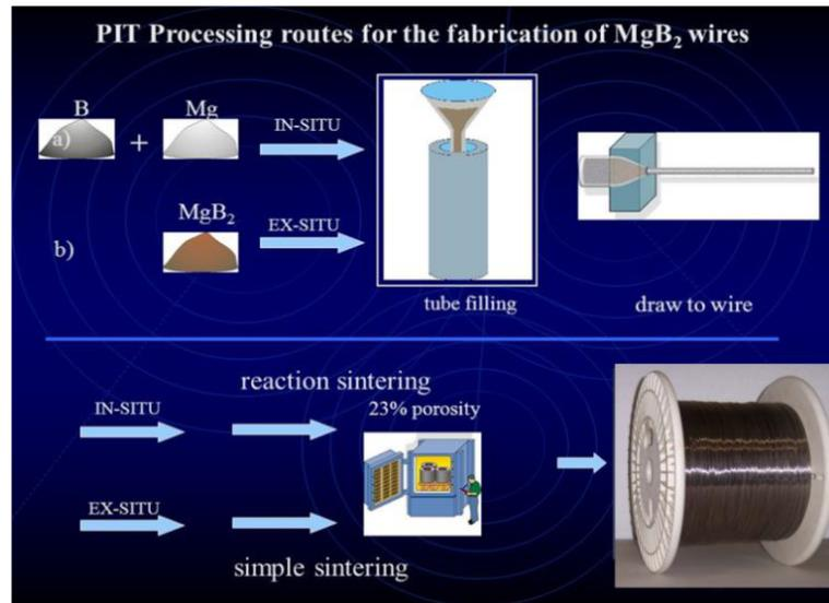
**Figure 2.6:** Fabrication steps for PIT  $MgB_2$  wire
