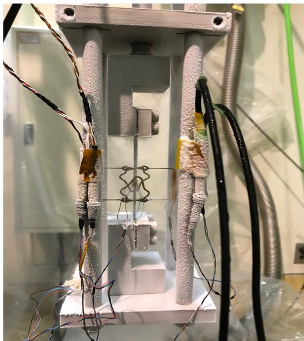
**Figure C.3:** RT and 77 K tensile test setup
