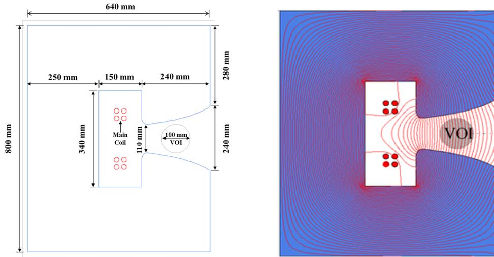
**Figure 2.3:** Cross section of combined function magnet
