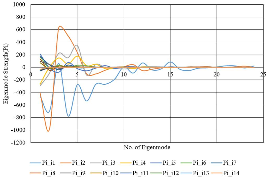
**Figure A.3:** Eigenmode strength as a function of number of eigen modes
