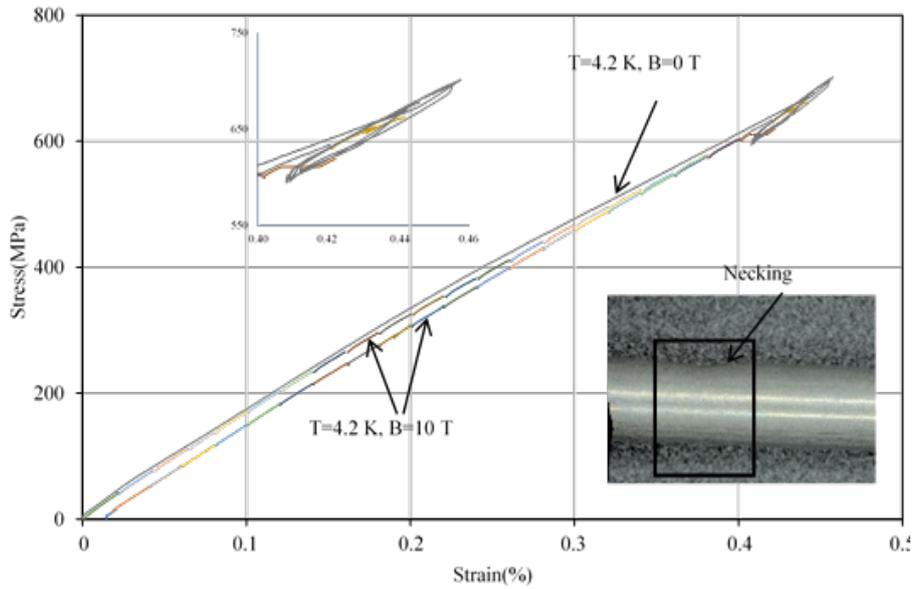
**Figure 4.19:** S-S curves at 4.2 K, under 0 T and 10 T magnetic field.
