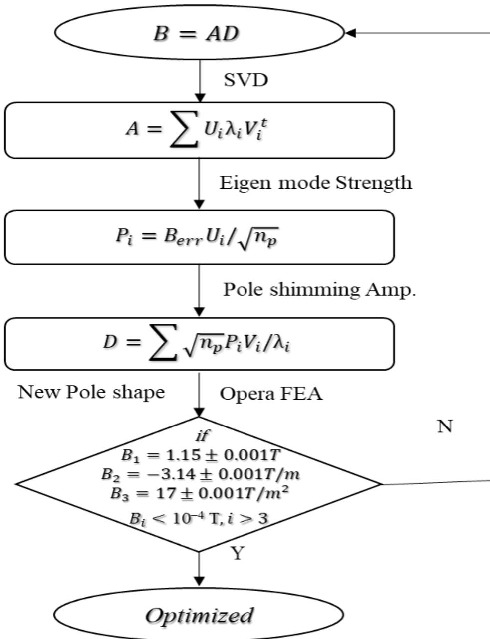
**Figure 3.8:** Singular value decomposition algorithm
