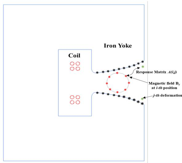
**Figure 3.2:** Geometry for shimming calculation
