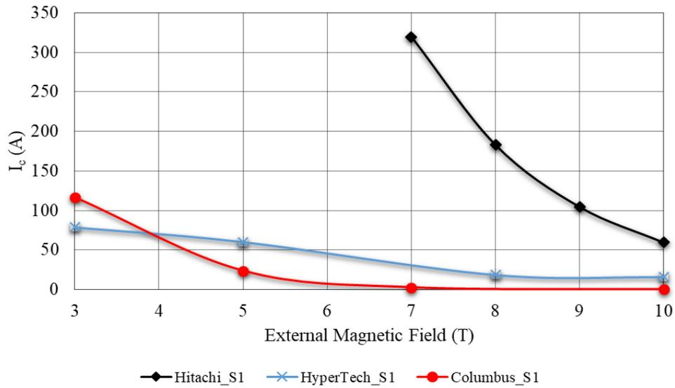
**Figure 5.2:** Comparison of  $I_c$  as a function of external magnetic field in three  $MgB_2$  wire with different composition
