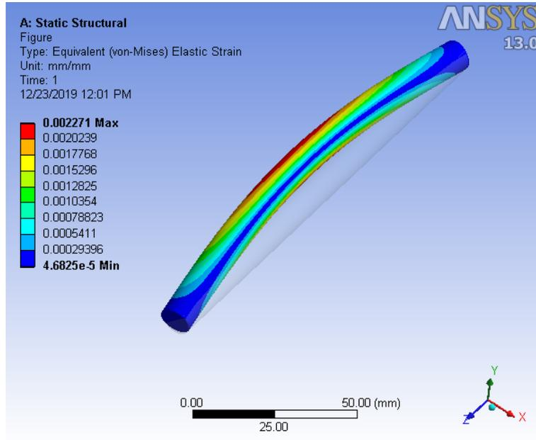
**Figure 4.8:** Strain distribution in 140 mm length cable.
