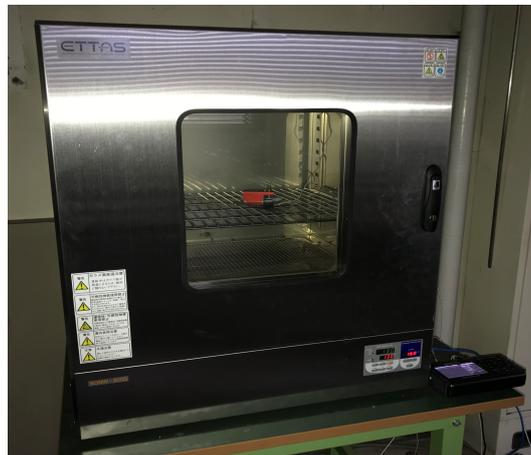
**Figure C.2:** Furnace for strain gauge bonding
