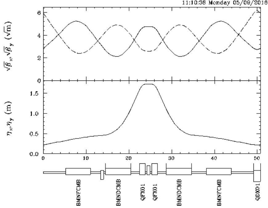
**Figure 2.2:** Beam optics of one arc module in the arc section of the stretcher ring
