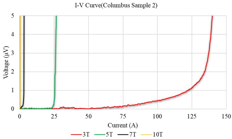
**Figure D.9:** Columbus sample 2 - I-V curve under variable field (3 T - 10 T) under 0 % strain
