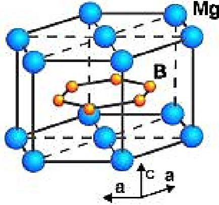
**Figure 2.5:** Crystal structure of  $MgB_2$
