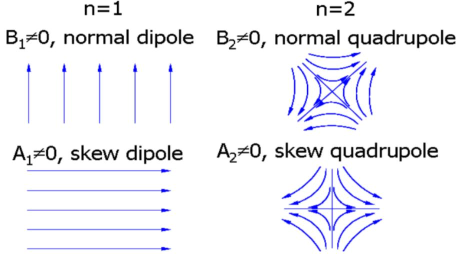
**Figure 3.1:** Field lines of normal and skew dipole and quadrupole magnets: (above-left): normal dipole field lines; (below-left): skew dipole lines; (above-right): normal quadrupole field lines; and (below-right): skew quadrupole field lines
