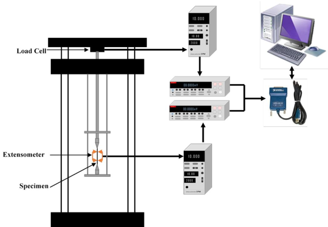
**Figure 4.11:** Schematic of tensile test setup at RT and 77 K
