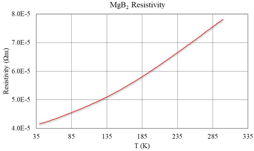
**Figure B.5:** Variation of resistivity of MgB<sub>2</sub> with temperature
