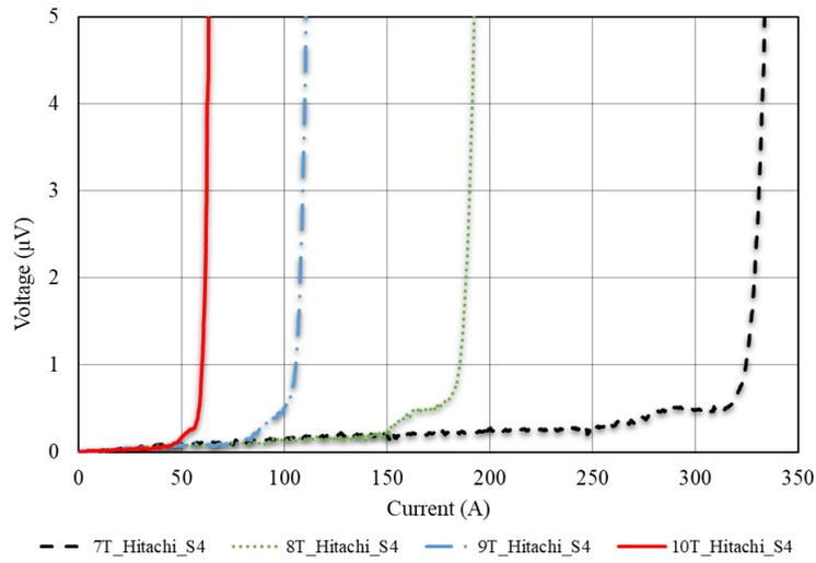
**Figure D.5:** Hitachi Sample 4 - I-V curve under variable field (7 T - 10 T) under 0 % strain
