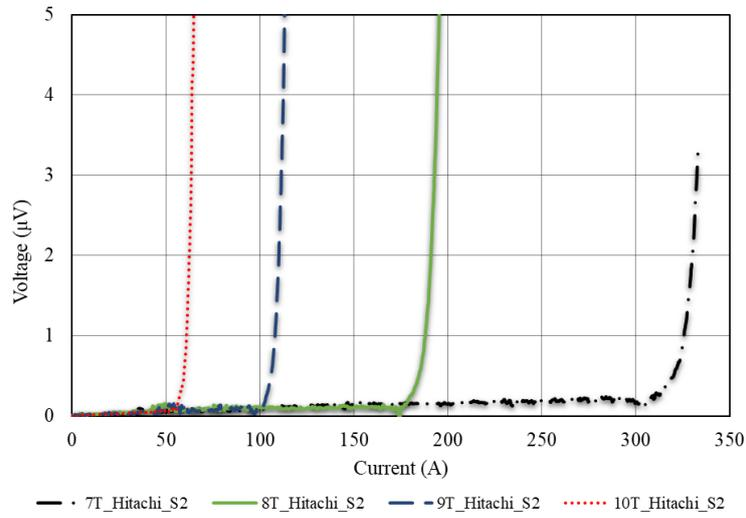
**Figure D.3:** Hitachi Sample 2 - I-V curve under variable field (7 T - 10 T) under 0 % strain
