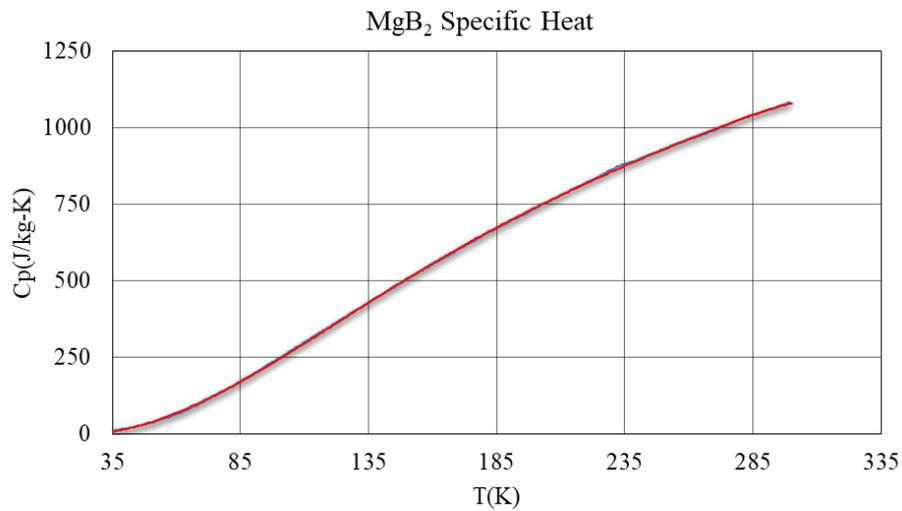
**Figure B.1:** Variation of specific heat of MgB<sub>2</sub> with temperature. [17]
