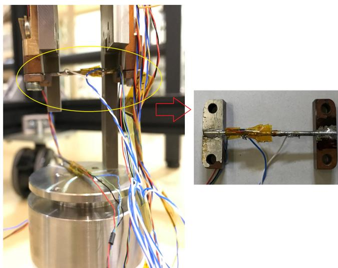
**Figure C.4:** 4.2 K test probe sample space
