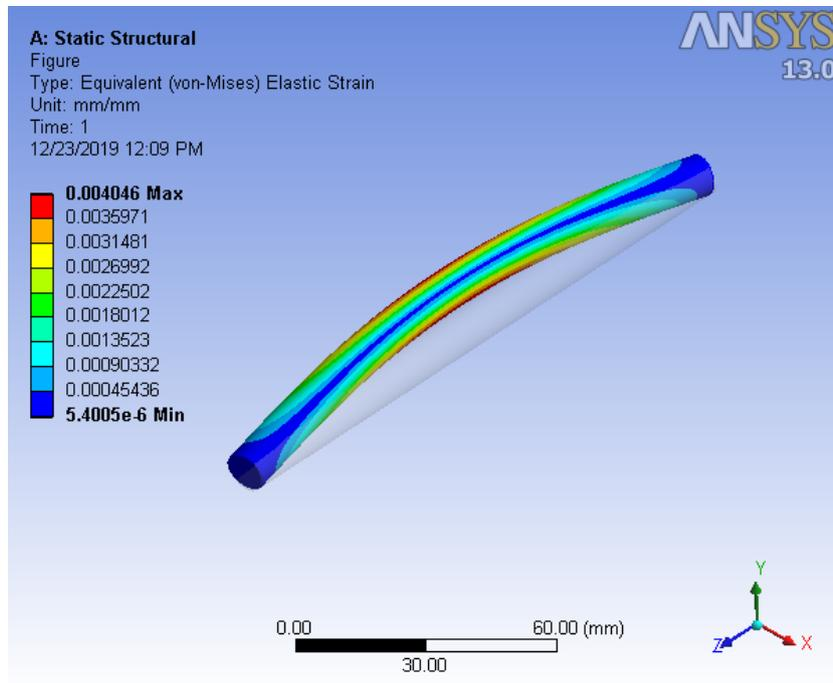
**Figure 4.9:** Strain distribution in 150 mm length cable.
