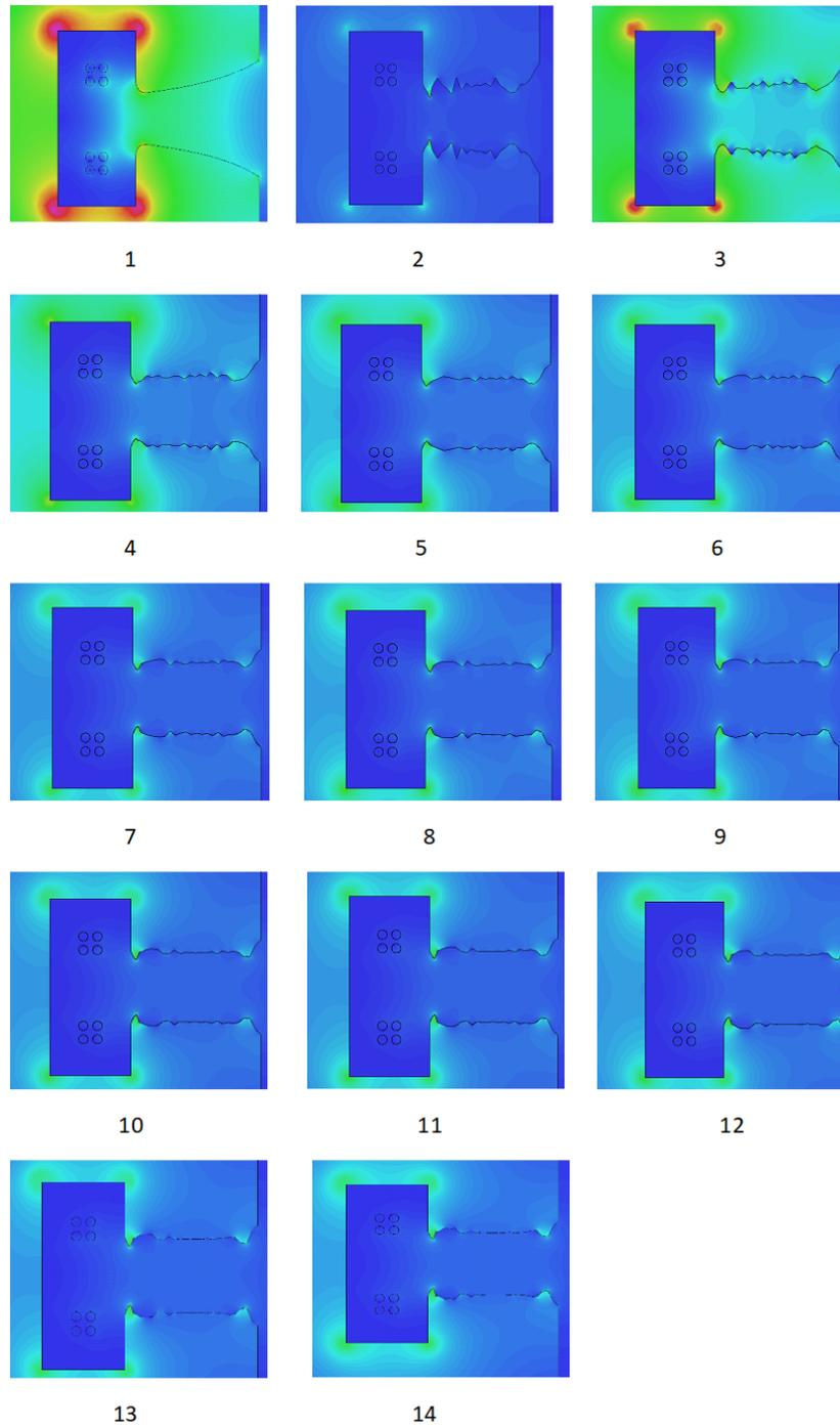
**Figure 3.7:** Iterative pole profile convergence combined function to dipole
