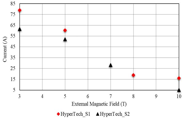
**Figure 4.16:**  $I_c$  as a function magnetic field for HyperTech  $MgB_2$  wire at 4.2 K
