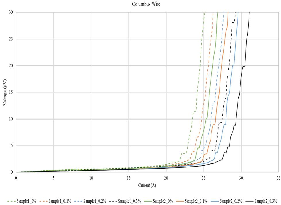
**Figure D.10:** Columbus samples - I-V curve under variable strain and fixed field  $B= 5 \text{ T}$
