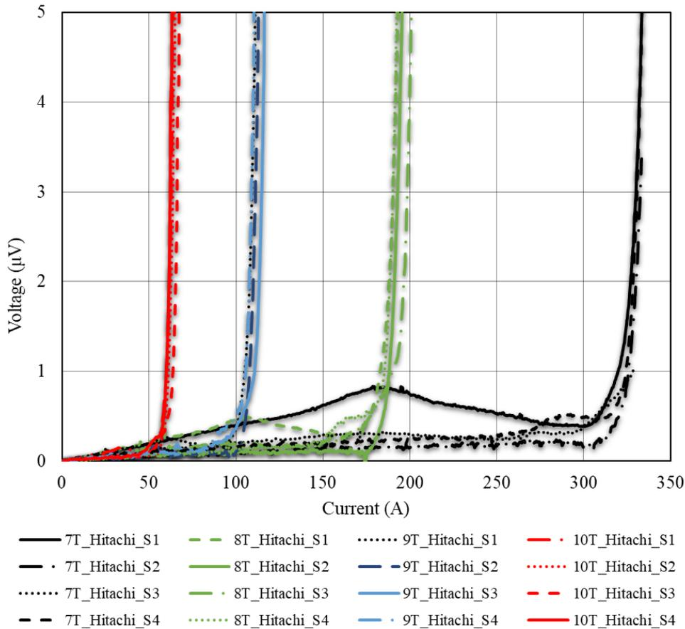
**Figure D.1:** Hitachi samples dependence of external magnetic field on critical current, strain = 0 %
