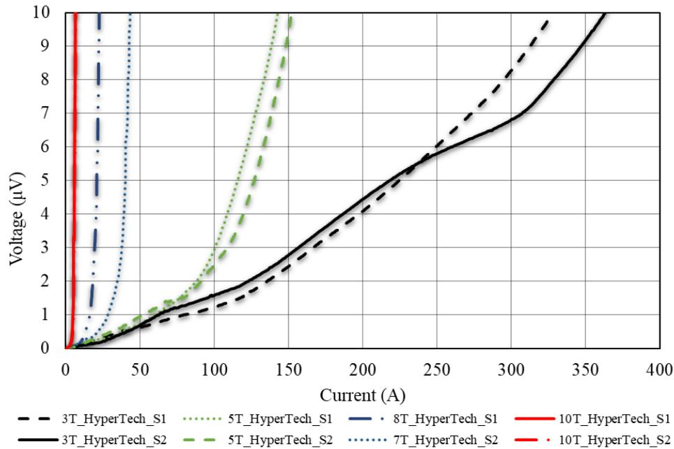
**Figure D.11:** HyperTech samples dependence of external magnetic field on critical current, strain = 0 %
