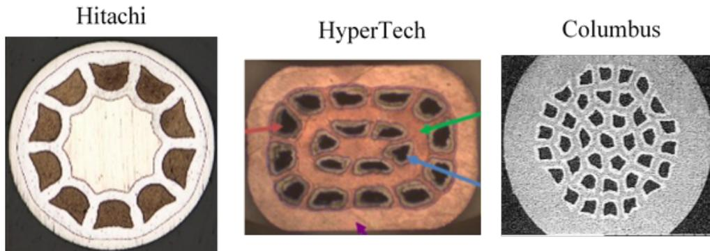
**Figure 4.10:** Cross-section view of Hitachi, HyperTech and Columbus sample wires
