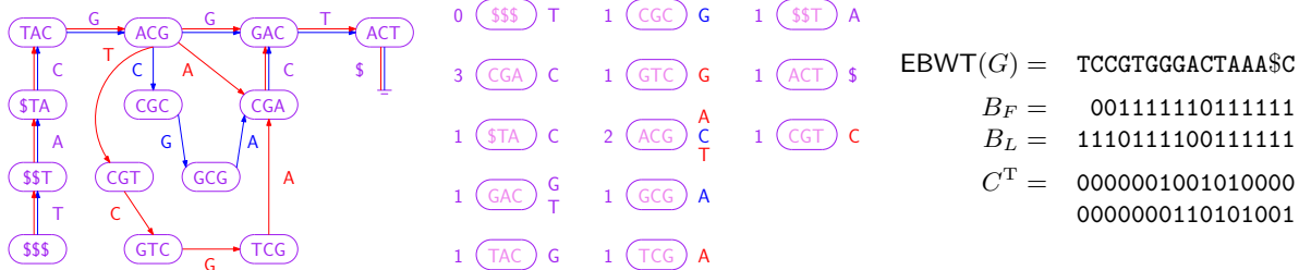
Figure 4.1: Left: A colored de Bruijn graph consisting of two individual graphs, whose edges are shown in red and blue. (We can consider all nodes to be present in both graphs, so they are shown in purple.) Center: The nodes sorted into co-lexicographic order, with each node's number of incoming edges shown on its left and the labels of its outgoing edges shown on its right. The edge labels are shown in red or blue if the edges occur only in the respective graph, or purple if they occur in both. Right: Our representation of the colored de Bruijn graph: the edge-BWT and bitvectors for the BOSS representation for the union of the individual graphs, and the binary array C (shown transposed) whose bits indicate which edges are present in which individual graphs.
