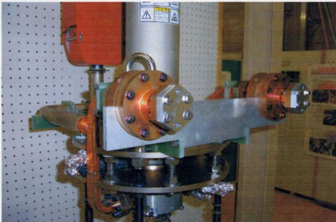
Figure 4.3.6: X-band travelling-wave window in the 75MW E3761 Toshiba klystron.
