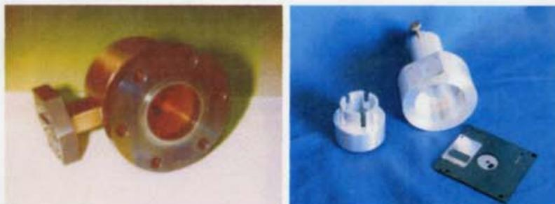
Figure A6.2: Wrap-around TE<sub>10</sub>-TE<sub>01</sub> mode converter
