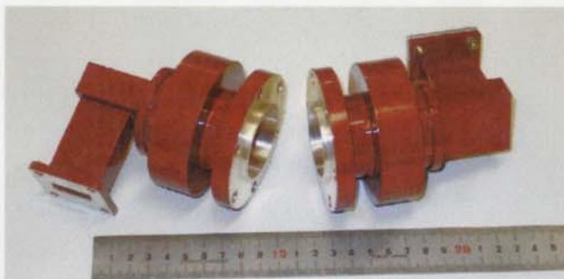
Figure A6.3: Choke TE<sub>10</sub>-TE<sub>01</sub> mode converter
