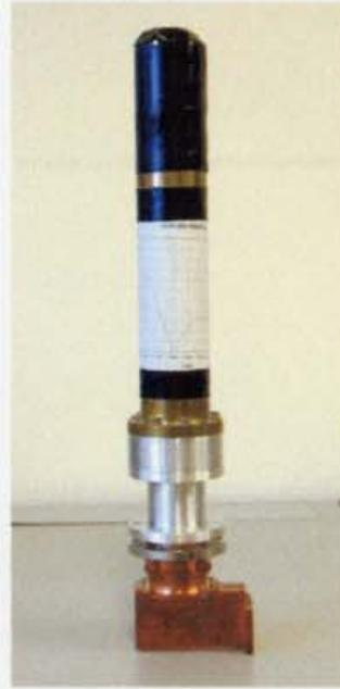
Figure 5.3.3: Converter, window, and load.
