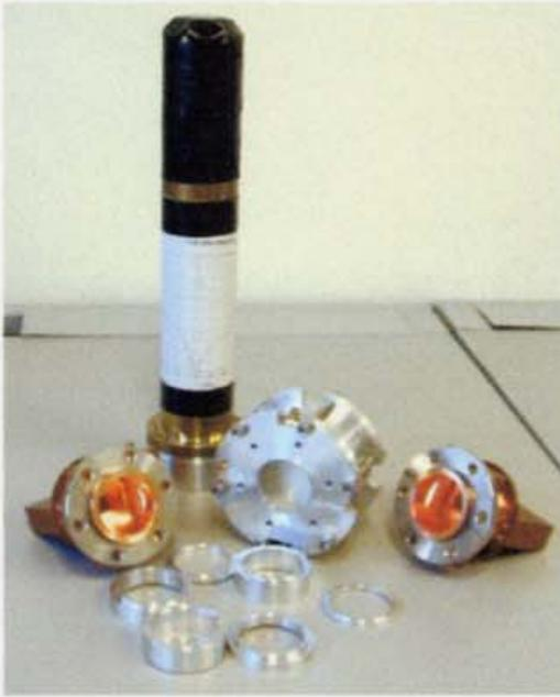
Figure 5.3.1: Low power elements: two converters, window, load, spacers.
