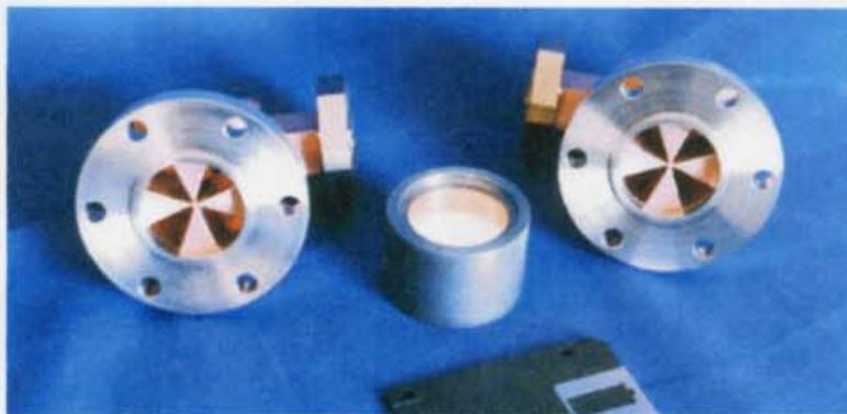
Figure A6.1: Cross TE<sub>10</sub>-TE<sub>01</sub> mode converter and window on its base.
