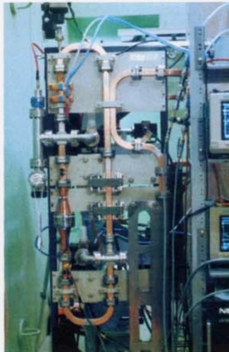
Figure 4.3.2: X-band resonant ring at KEK.
