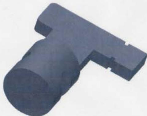
Figure A6.6: Iris TE<sub>10</sub>-TE<sub>01</sub> mode converter
