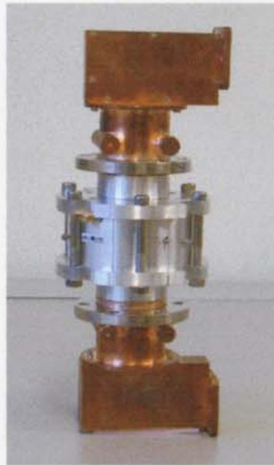
Figure 5.3.6: Window together with two converters. Parallel position
