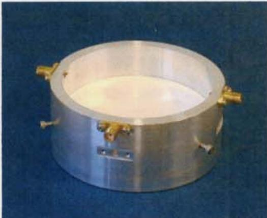
Figure 5.3.2: Ceramic unit with antennas.
