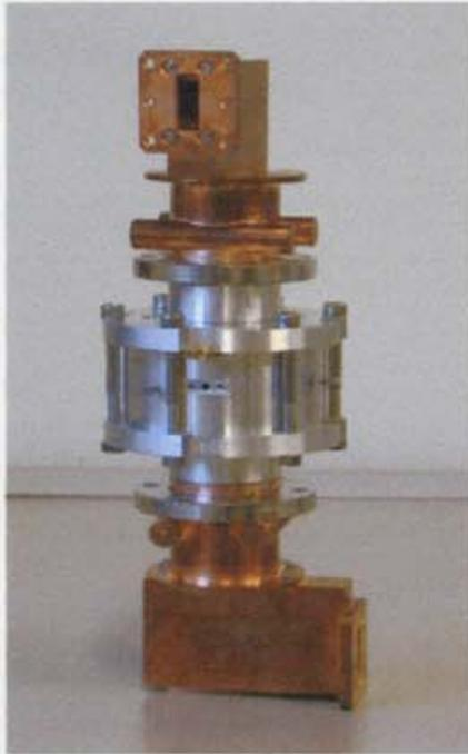
Figure 5.3.5: Window together with two converters. Orthogonal position.
