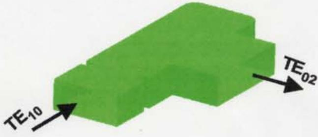
Figure 5.2.8: Junction of rectangular waveguides transforms  $TE_{10}$  mode to  $TE_{20}$  mode.
