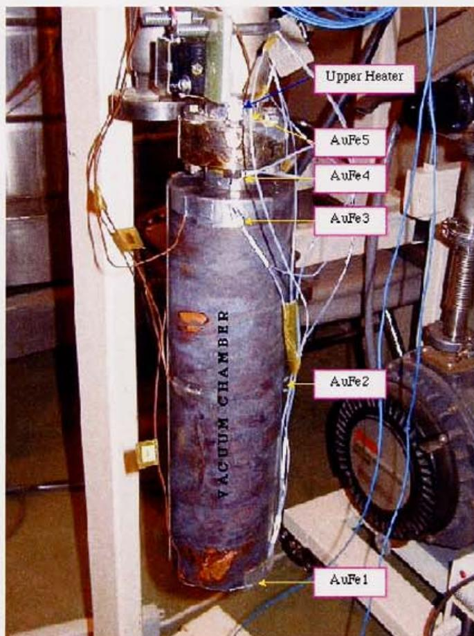
Figure 2.3: Photograph of our designed vacuum chamber. This photograph was taken after baking at  $150^{\circ}\text{C}$  in ambient air. So, its outside surface turned ash color.
