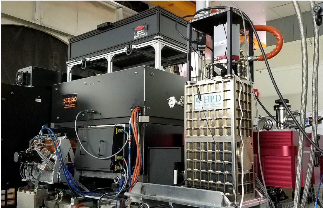
Figure 4.2 The SCExAO instrument with its science modules: CHARIS (the red box in the right), MEC (the silver tower in the left end), Visible bench on the top. Picture Courtesy: https://www.naoj.org/Projects/SCExAO/
