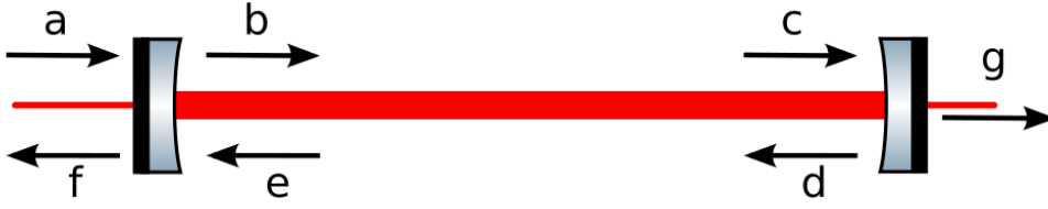
Figure 2.4: Fabry-Perot cavity. Different arrow marked with alphabet 'a' to 'g' indicates different fields amplitude. These fields are electric fields, the square of them corresponds to power. We could also see that the red line which represents the laser light is thicker inside the cavity which means the light is stored inside the cavity and the power is enhanced.
