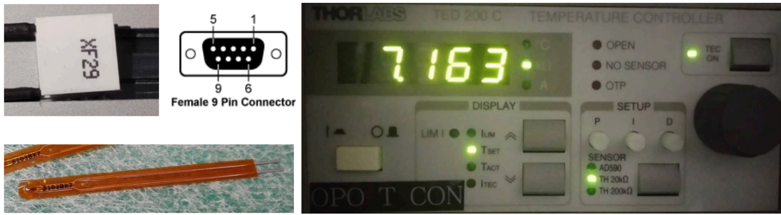
Figure 4.25: Left upper corner: Peltier. Left lower corner: thermistor. Upper middle: 9-pin layout for TEC200C. (connection assignment: 2-thermistor +, 3-thermistor -, 4-Peltier +, 5-Peltier -) Right: TEC200C front panel
