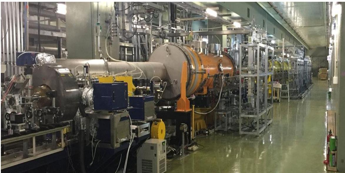
Figure 2-4: ILC cryomodule testing at the STF facility.
