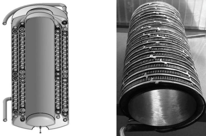
Figure 1-12: Coil-Finned 2K heat exchanger for vertical test cryostat at XFEL, DESY [16].
