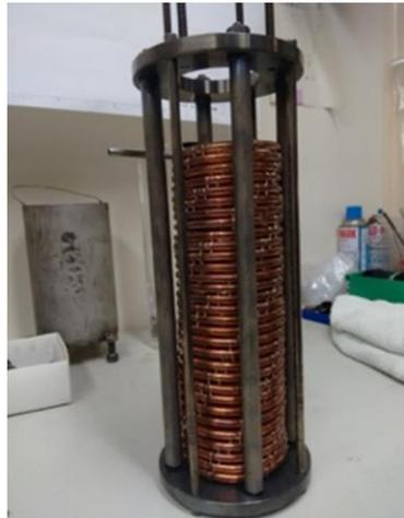
Figure 2-9: Cross section of the 2K HX\_1 (on the left) and its helically coiled tube (on the right).
