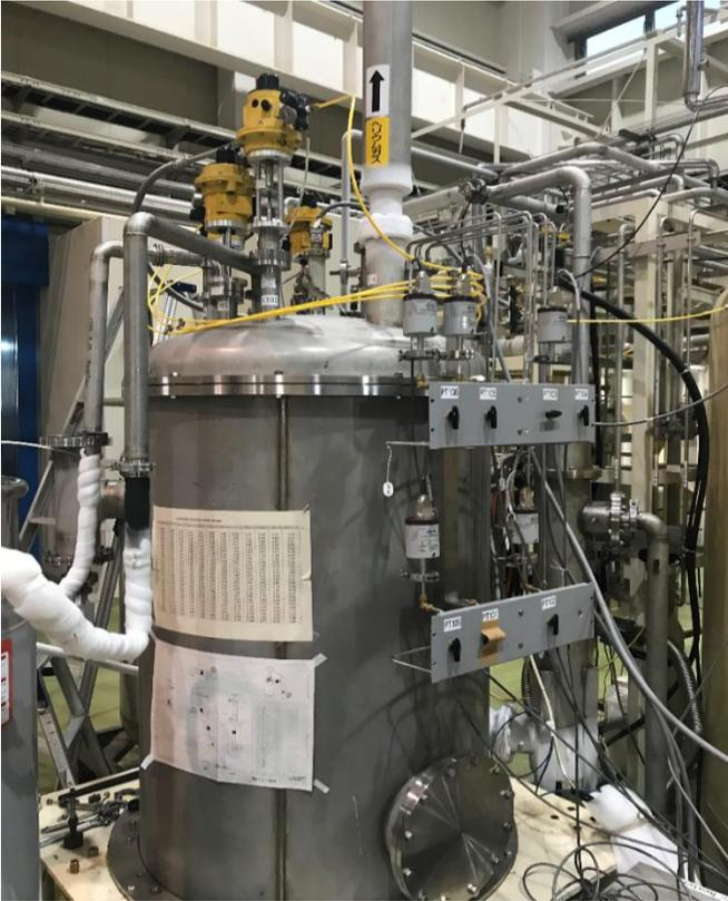
Figure 6-4: 2K Cold box for the heat exchanger test stand.
