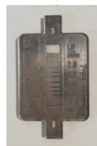
MTF type 14 Pb thickness: 0.03 mm Spatial frequency: 2.0 to 20 lp/mm
