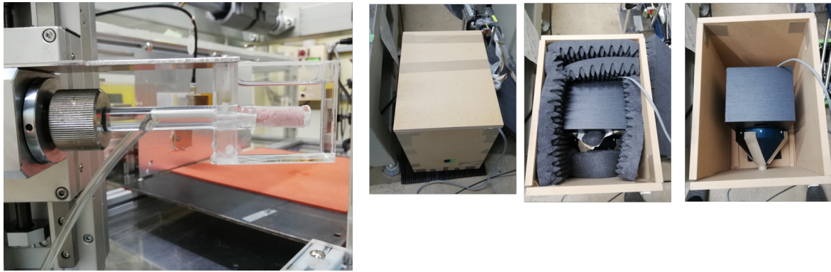
Fig. 8.14. Photos of X-ray elastography setup by air pressure. (Left) Fixed sample. (Right 3 photos) Inside and outside of the soundproof box. A speaker was surrounded by insulation materials.
