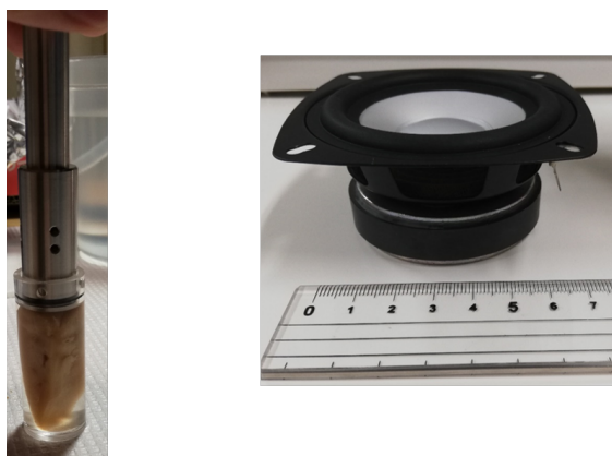
Fig. 8.16. Photos of jigs for elastography by air vibration (Left) and a small speaker (Right).
