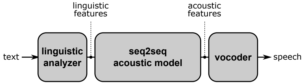
Figure 2.9: A conceptual representation of a seq2seq TTS pipeline.
