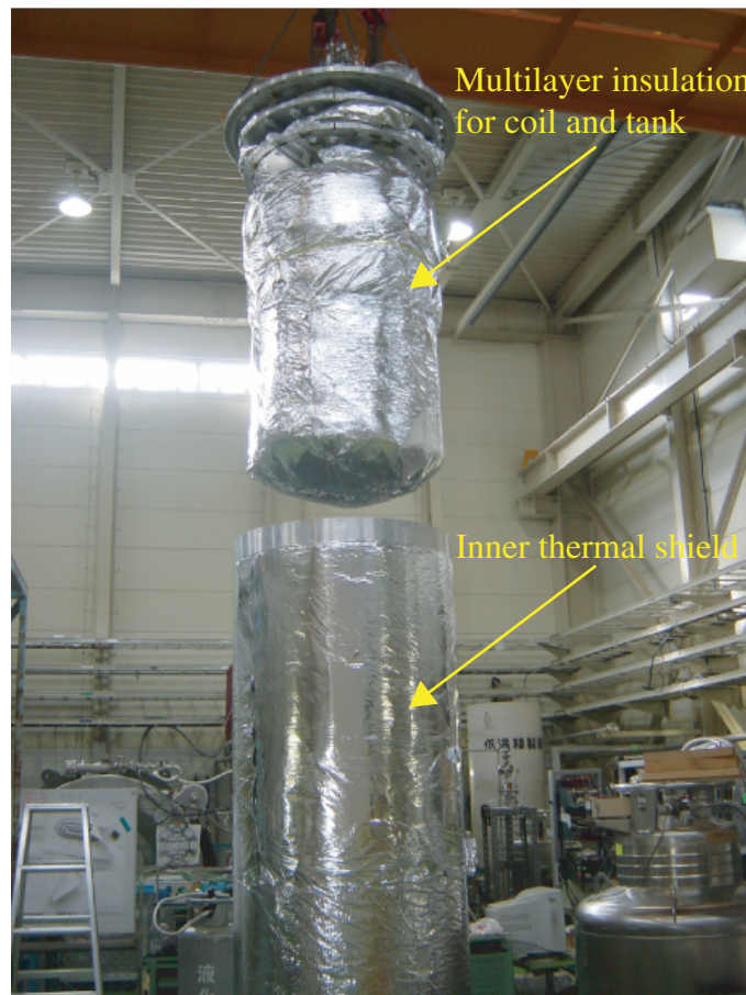
Figure 58: Thermal shield for prototype coil and reservoir tank
