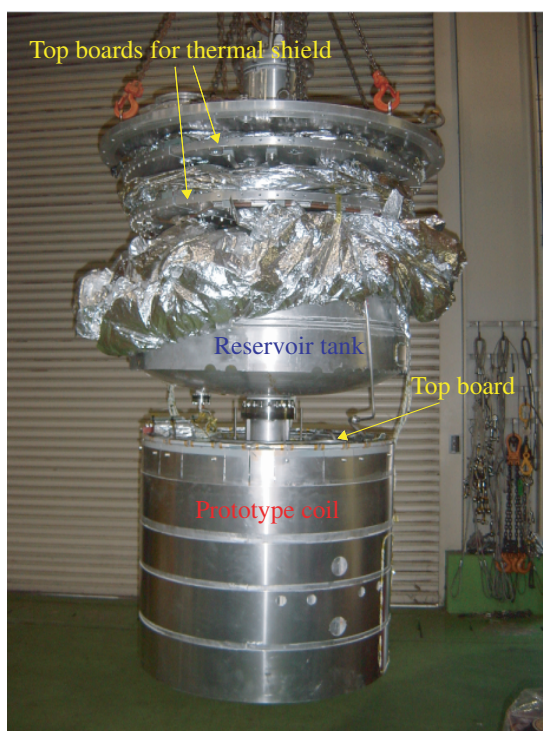
Figure 56: Prototype coil suspended in vertical position
