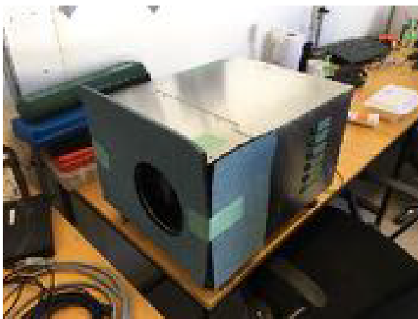
Figure 3.14: Coherent source for checking band and polarization angle.
