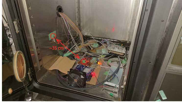
Figure 5.21: Laboratory setup to measure temperature difference between the mezzanine board and the neighboring wall.
