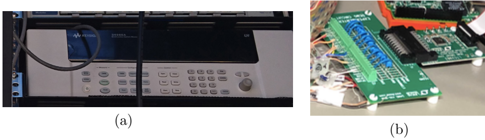
Figure 5.2: Images of temperature measuring instruments. (a) 34980A. (b) LTC2983.
