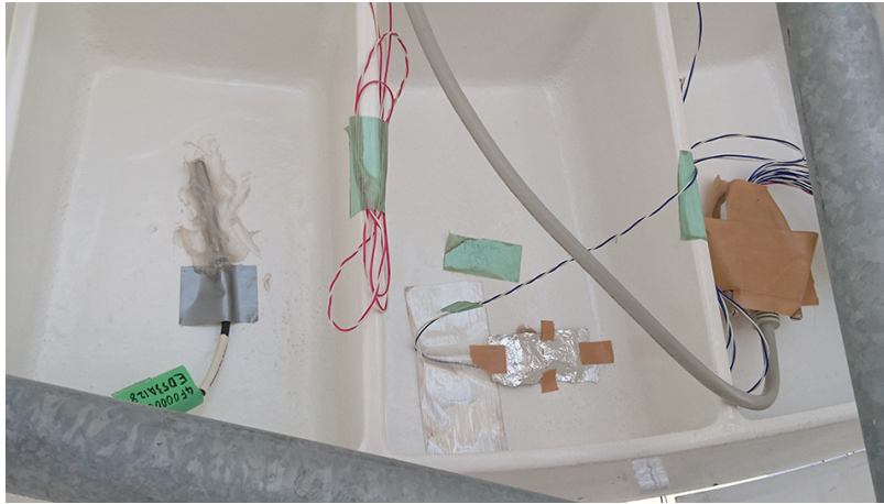
Figure 5.8: Photo of a sun-shaded thermistor attached on the bottom of back of the primary mirror. An onewire sensor is at the left of the thermistor for cross check of absolute temperature.
