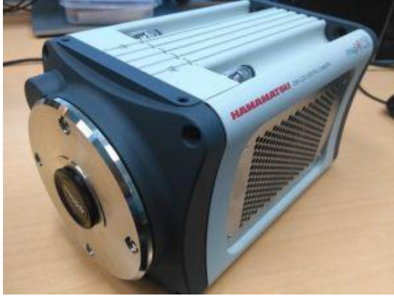
Figure 2-3: EMCCD camera (ImagEM X2 C9100-23B, Hamamatsu Photonics)
