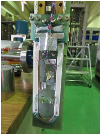
Fig. 2-12 Hall probe installed on the sample holder.
