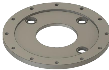
Figure 4.4 Top flange of vacuum chamber
