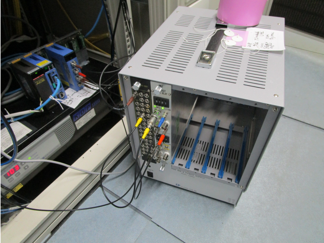
FIGURE 6.3: The test bench of prototype read-back system with a dummy signal. NIM modules are used to provide a “Trig-in” signal to the TS module.
