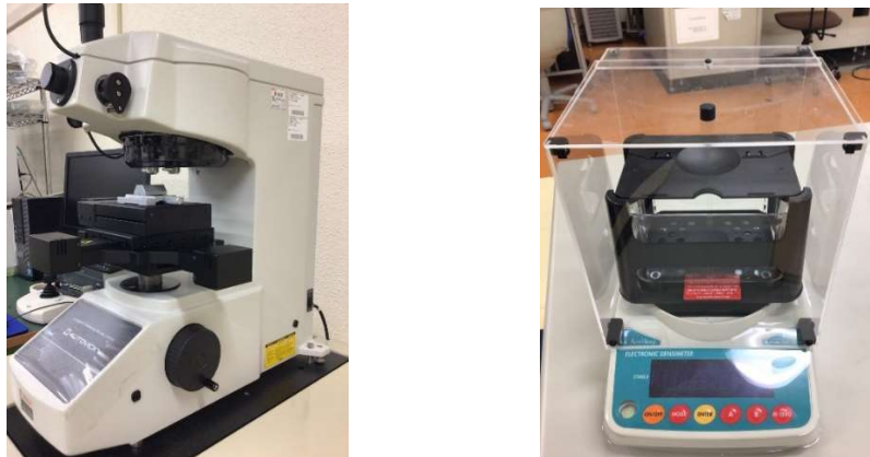
Figure 2.4 The pictures of Vickers hardness machine and densimeter.
