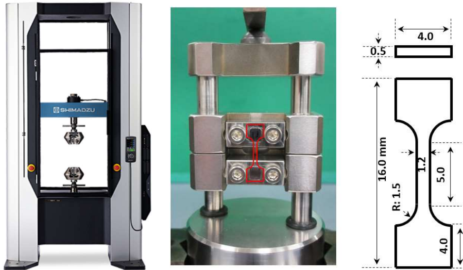
Figure 5.3.2 images of the tensile machine, tensile test fixture and the tensile sample.
