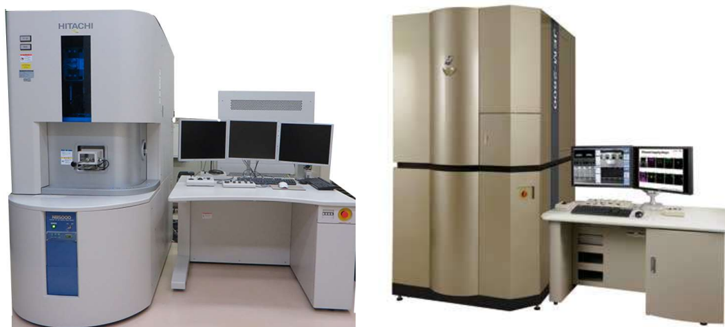
Figure 4.2 Images of the FIB and TEM machines.
