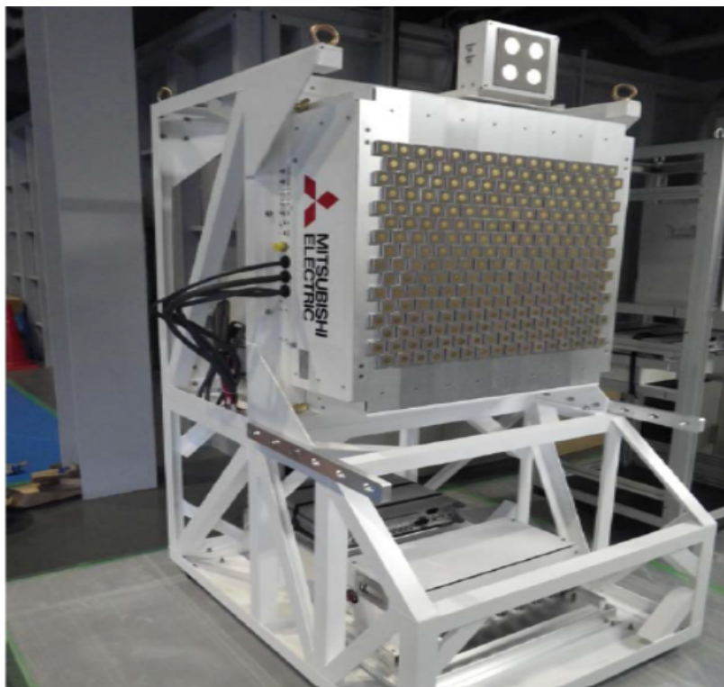
FIGURE 2.14: Phased array model by Kyoto Uni.
