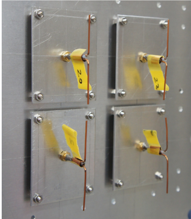
FIGURE 3.26: 2x2 dipole Antenna Array without Deformation.
