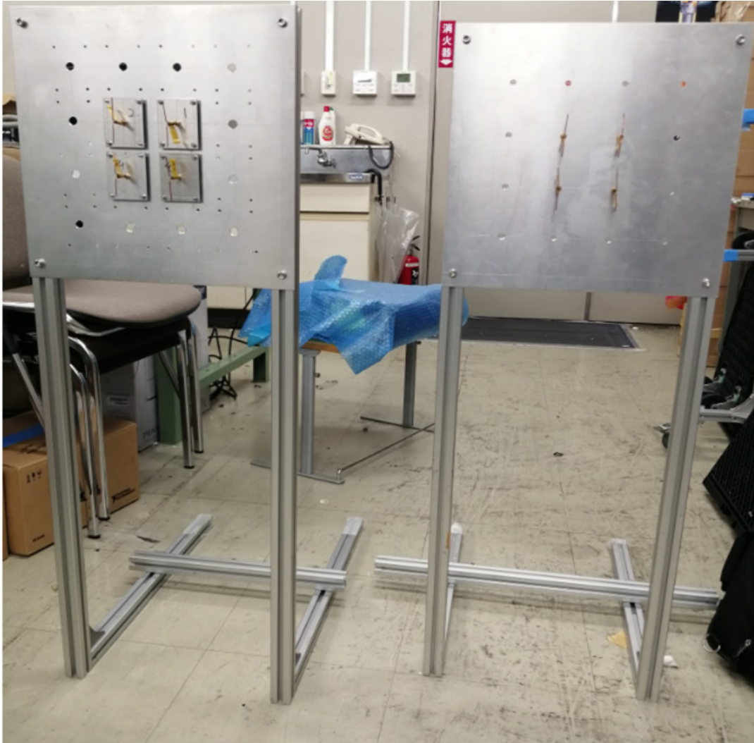
FIGURE 3.29: 2x2 dipole Antenna Array with whole antenna Deformation.
