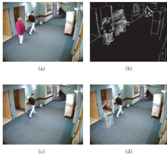
Fig. 2.11 Example of obscuring people: (a) original image, (b) edge motion history image, (c) original image restored but with woman in pink shirt removed, (d) final obscured image (reprinted from Chen et al. [5]).
