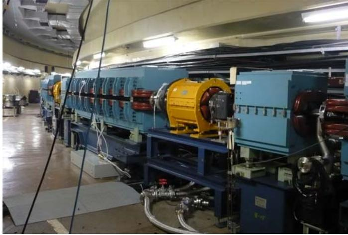
Fig. 5. KEK-12 GeV proton synchrotron ring composition
