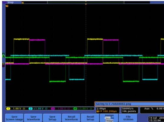
Fig. 75. (c) Output from the induction acceleration control system at 100  $\mu$ sec from the start. Long pulse generation in Stage I together with the set signal (pink and yellow) and the reset signal (blue and green).
