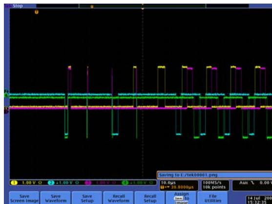
Fig. 75. (b) Output from the induction acceleration control system in the early acceleration region of Stage I, together with the set signal (pink and yellow) and the reset signal (blue and green).
