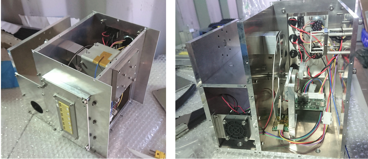
Figure 40: Photos were taken during assembly in the laboratory. (Left) top panel and service window are taken off. (Right) A connector panel is removed. In addition, outer and inner heater covers are removed to show the heater structure.
