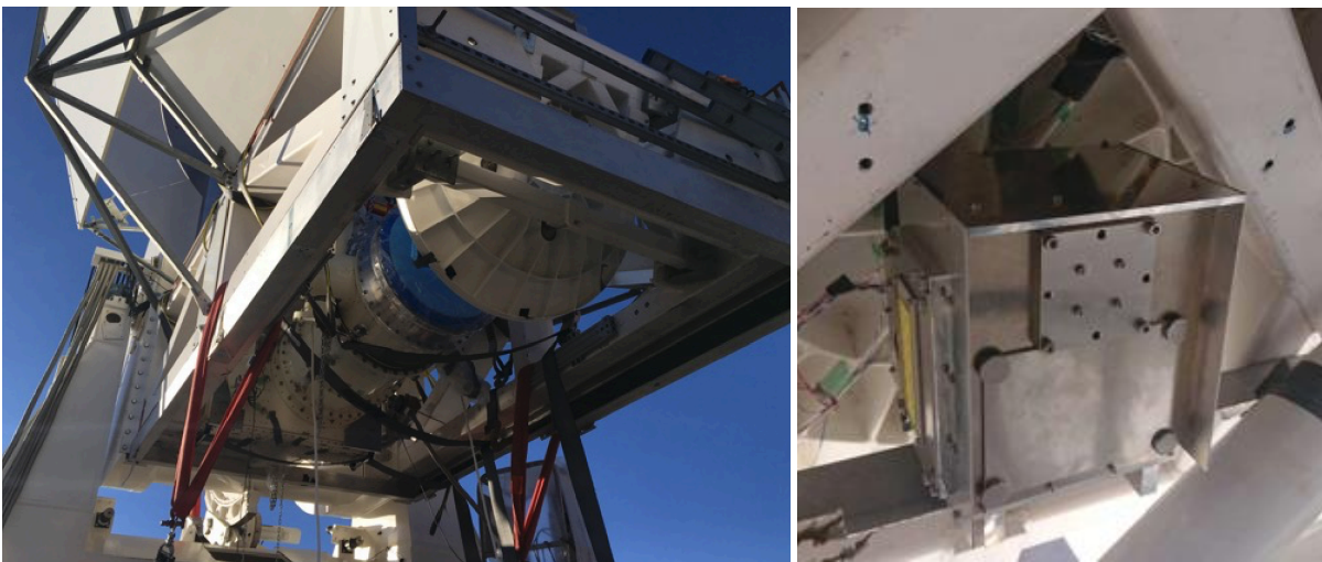
Figure 35: The PB-2 receiver installed to the telescope (left) and the stimulator installed in the back of the secondary mirror (right).
