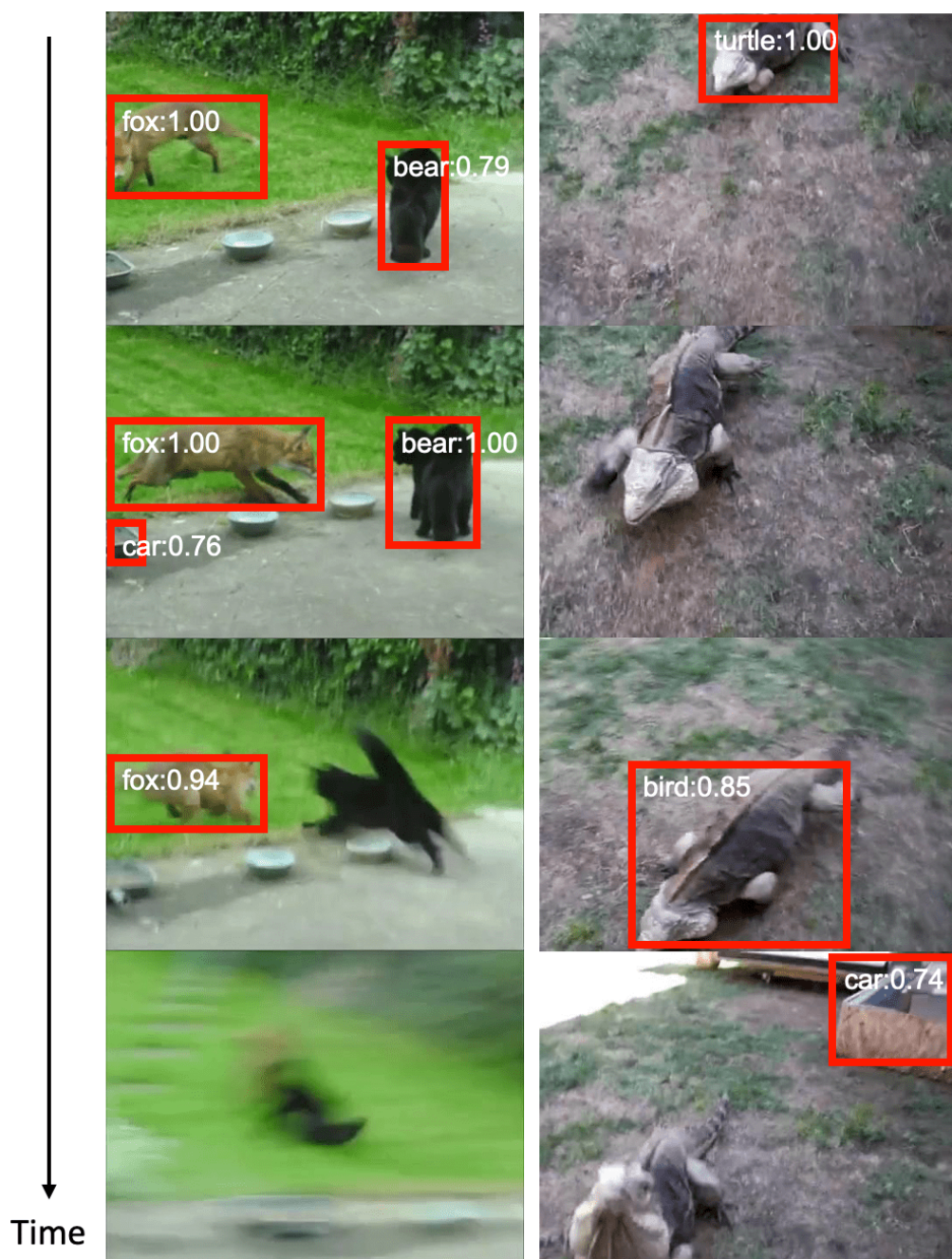
Figure 1.2: Examples of false-negative and false-positive detection with Faster R-CNN due to apparent changes with time. The changes cause the problems, such as detecting an object that is not the target of detection or failing to detect an object in a scene that should be detected.
