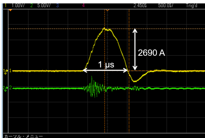
FIGURE 7.24: Screenshot of the oscilloscope in the current excitation test with a 1 \mu s pulse width.
