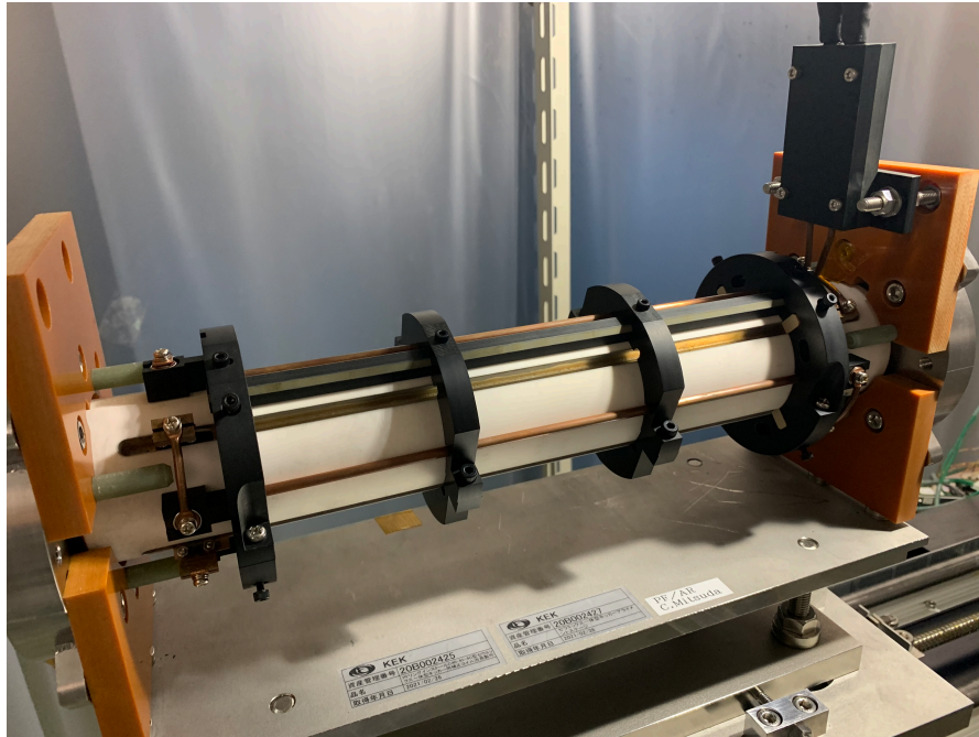
FIGURE 7.4: Assembly of the octupole CCiPM.
