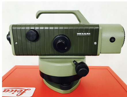
FIGURE 3.11: Wild N3 for alignment in the vertical direction.
