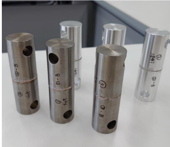
Figure 4-15: Samples for adhesive strength measurement
