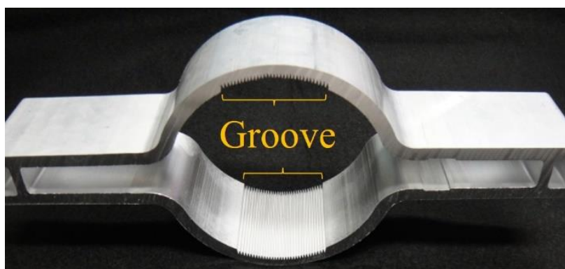
Fig. 1-7: Al-alloy groove surface without coating in the SuperKEKB
