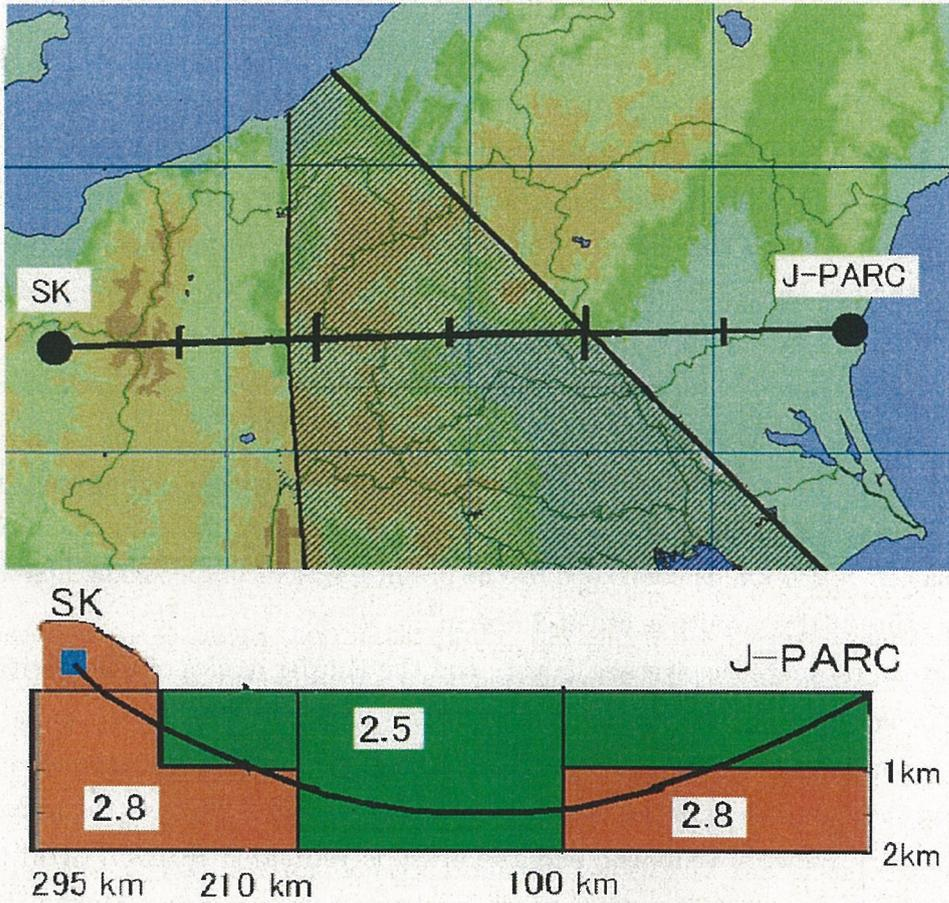
Figure 22: Upper: The Tokai-to-Kamioka baselines. The scale on the baseline shows the distance from J-PARC. The each interval corresponds to 50 km. The shadow region is Fossa Magna region [33]. Lower: The cross section view of the T2K experiment. The horizontal line shows the distance from the J-PARC and the vertical axis means the depth from the sea level. The number of each region means the average density. The unit is  $\text{g}/\text{cm}^3$ .
