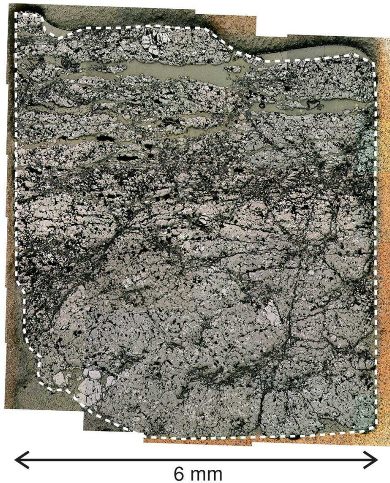
Figure 2.3: Reflected-light micrograph of specimen i01. The upper base is the crater floor. The homogeneous gray areas in the upper half of the specimen are epoxy-filled cracks.
