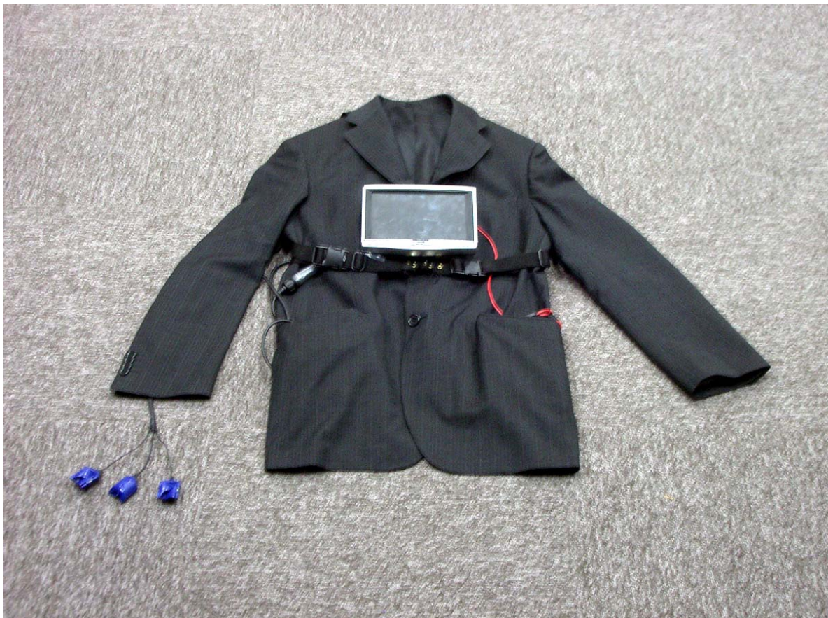
Illustration 4.5: Wearable system – Second enhanced jacket, with screens and biosensors.
