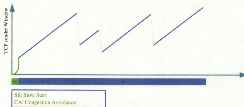
Figure 6.1: Burst loss indication by receiving triple-duplicate acknowledgments
