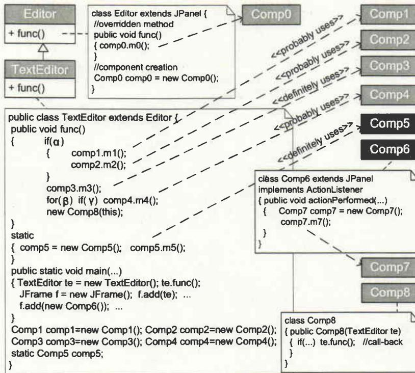
Figure 4.2: UML(51) class diagram of an example Java program that contains fundamental programming patterns
