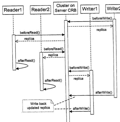
Figure 2.4: UML (51) sequence diagrams showing SOOM's consistency protocol operations. ("CR" stands for critical section.)
