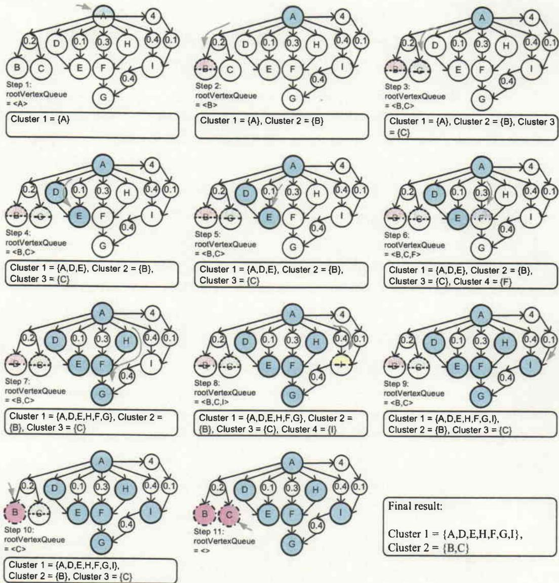
Figure 4.8: An example of intermittent delay-centric cluster identification
