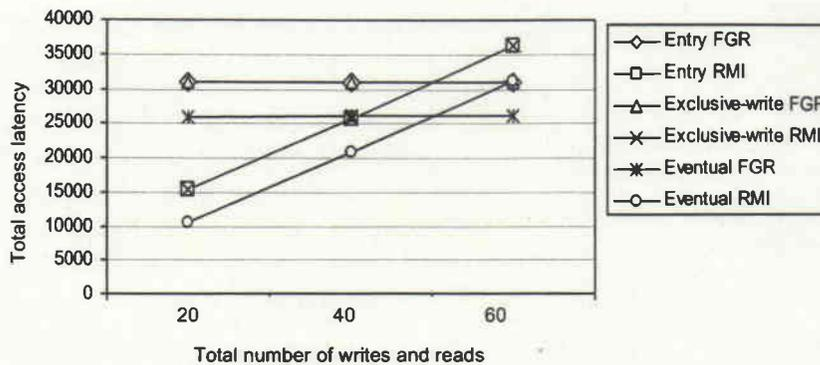
Figure 2.9: RMI and FGR cost comparison.
