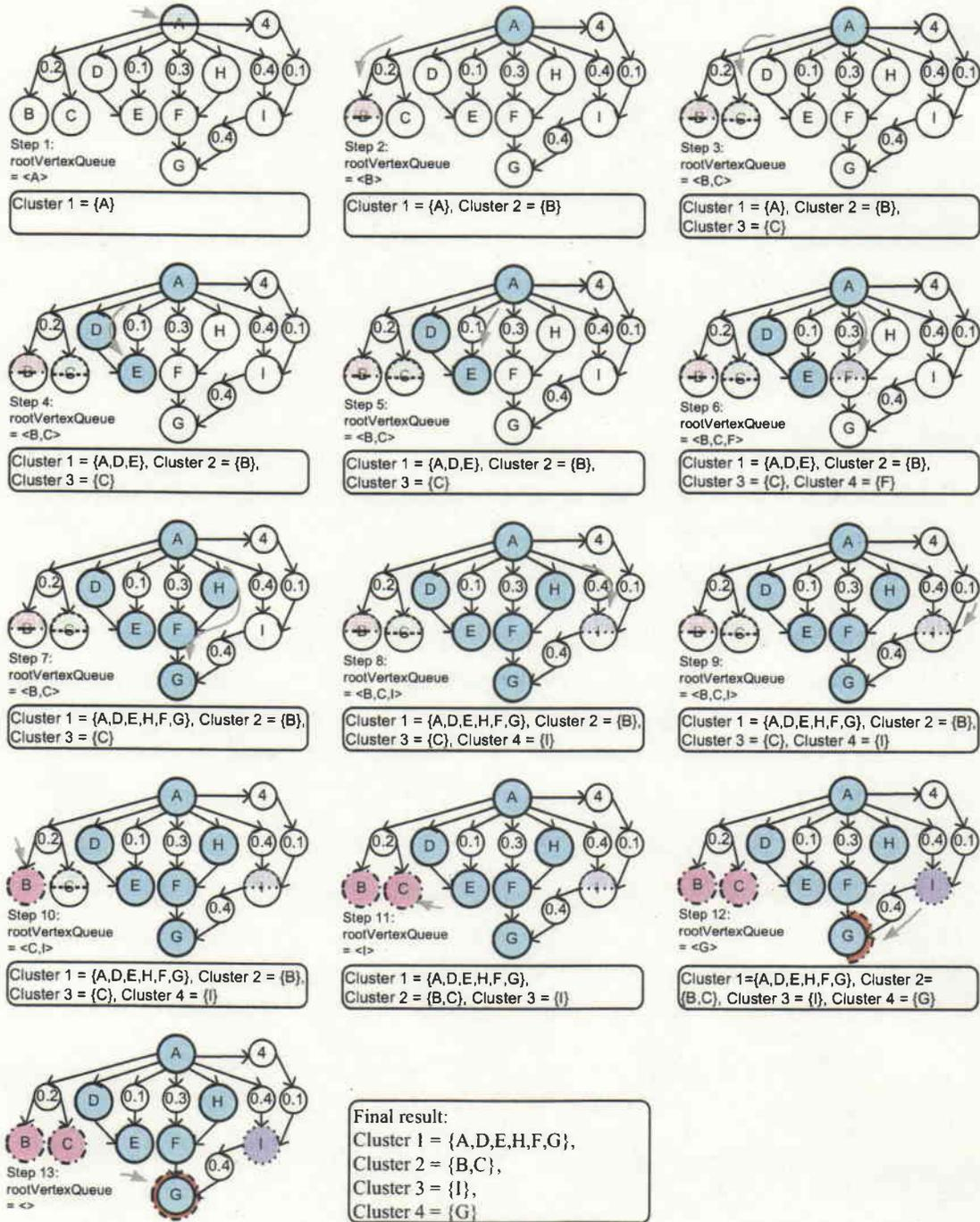
Figure 4.6: An example of initial delay-centric cluster identification
